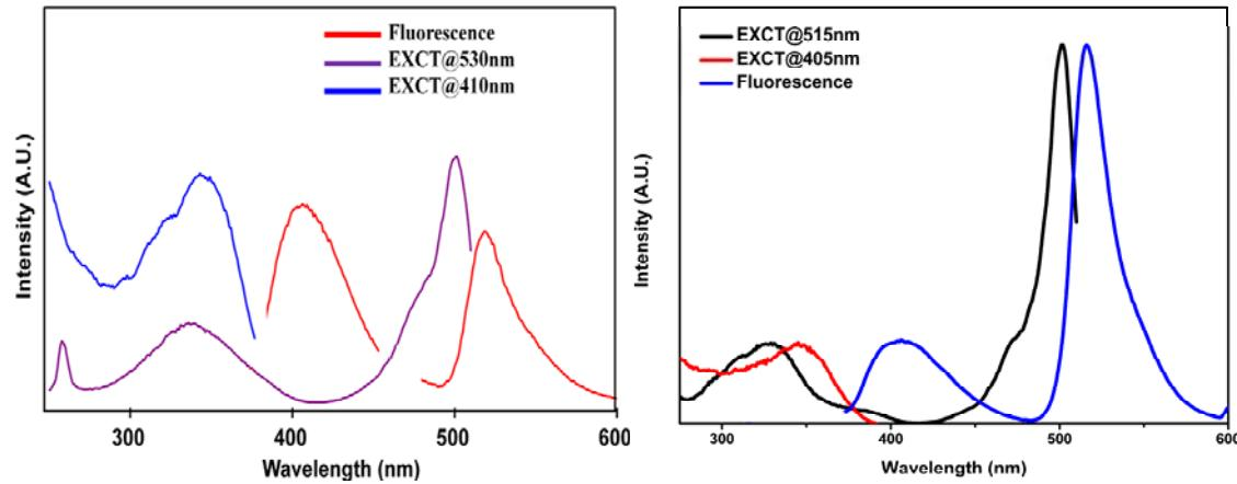
Figure S3: Fluorescence emission and excitation spectra for **2** (left) and **3** (right) ( $1\mu\text{M}$  in DCM)
