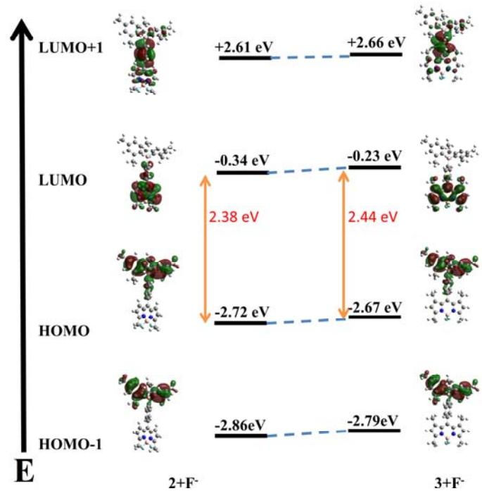
**Figure S19:** Comparison of electronically important MOs (Isovalue 0.02) of **2+F<sup>-</sup>** and **3+F<sup>-</sup>** (*Schematic: Not to scale*)
