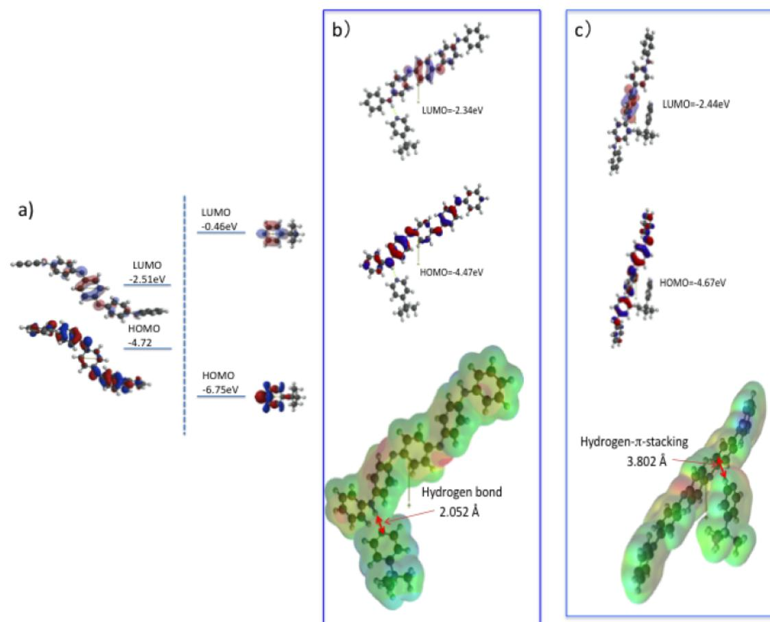
**Figure S4** Energy relationship and shape of the frontier orbitals of EPAT, TBP (a) and energy structures of two kinds of associated EPTA and TBP, and electrostatic potential map and specific distances for the associated EPAT/TBP molecules through hydrogen bonding (b) and through weak hydrogen- $\pi$  stacking bond (van der Waals bond) (c).
