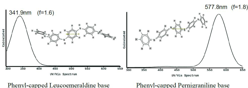
**Figure S3** Simulated absorption spectra of the phenyl-capped aniline tetramers of leucoemeraldine base and a pernigraniline base determined by DFT calculations. The peaks corresponding to calculated intensity are very consistent with the experimental data. All quantum chemical calculations were performed using DFT at the B3LYP/6-31G(d) level with Spartan '10 package (Wavefunction, Irvine, CA).
