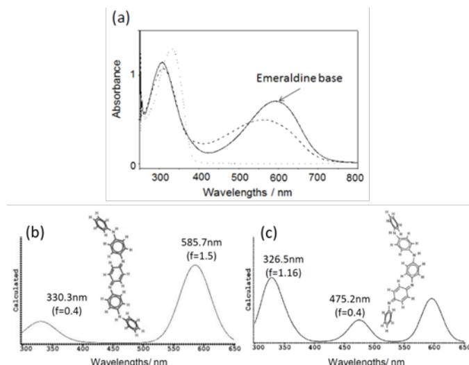
**Figure S2** Absorption spectra of phenyl-capped aniline tetramers for four structures, dot: leucoemeraldine-type (LPAT), solid: emeraldine-type (EPAT), dash: pernigraniline-type (PPAT) in DMF solution (a), the DFT-simulated absorption spectra of symmetrical EPAT (b) and
