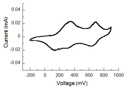
**Figure S1** A cyclic voltammogram of 1M  $\text{H}_2\text{SO}_4$  solution of EPAT. The scanned potential started from 0.9 V to  $-0.2$  V versus saturated  $\text{Ag}/\text{AgCl}$  reference electrode at the scan rate of  $100 \text{ mV s}^{-1}$ .
