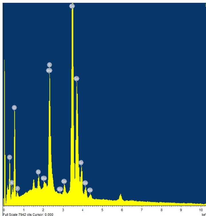
**Fig. S3** X-ray energy dispersive spectroscopy of MoS<sub>2</sub>/GNS CE.
