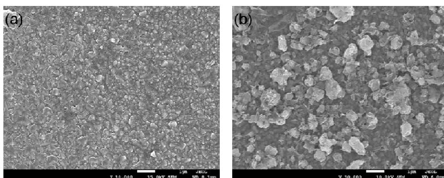
**Fig. S2** (a) before and (b) after the electrophoretic deposition of MoS<sub>2</sub>/GNS on a FTO substrate
