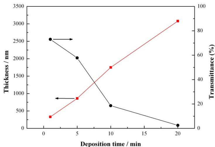
**Fig. S6** The relationship between the deposition time and the corresponding film thickness and transparency of MoS<sub>2</sub>/GNS CE. The transparency was measured at the wavelength of 550 nm. Each result was the average of three different MoS<sub>2</sub>/GNS CEs.
