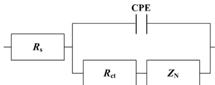
**Fig. S5** Equivalent circuit used for fitting the EIS results of the symmetric cells.
