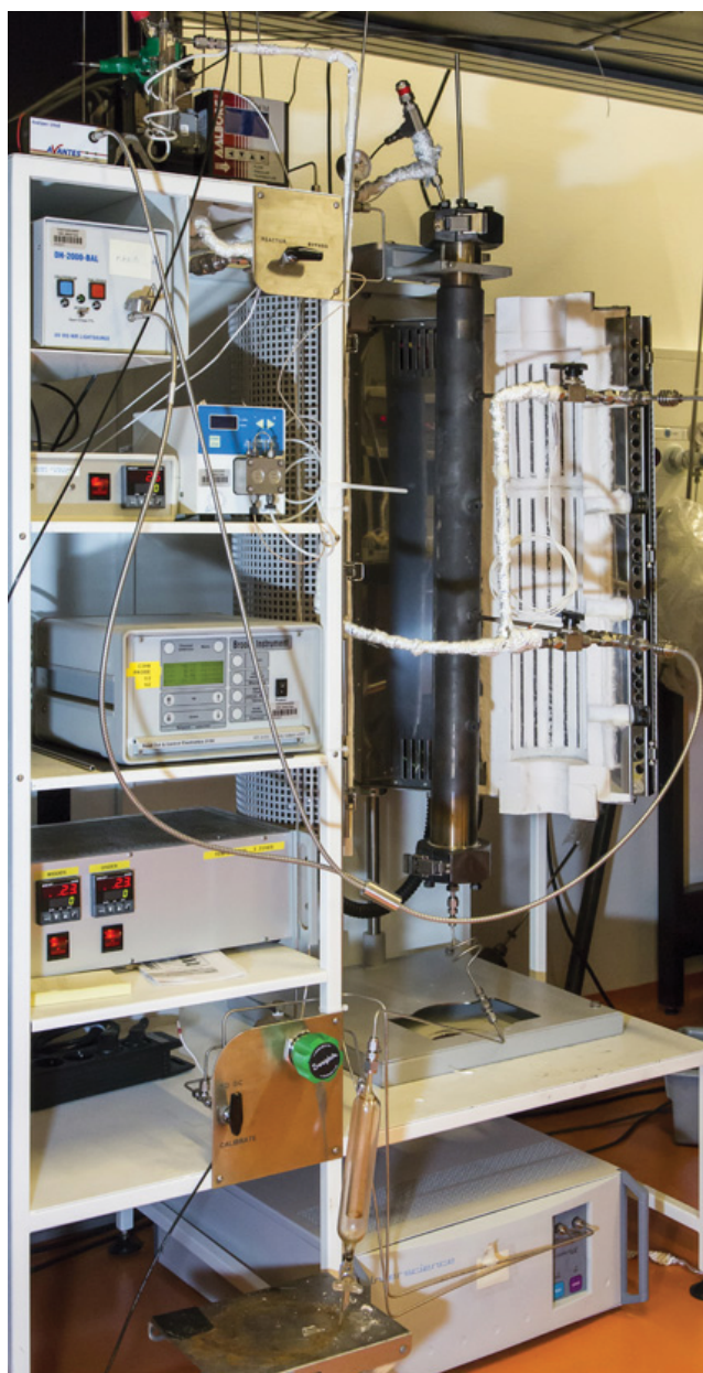
Fig. S1. Photograph of the pilot-scale reactor set-up developed for performing operando UV-Vis spectroscopy on catalyst bodies under realistic reaction conditions.
