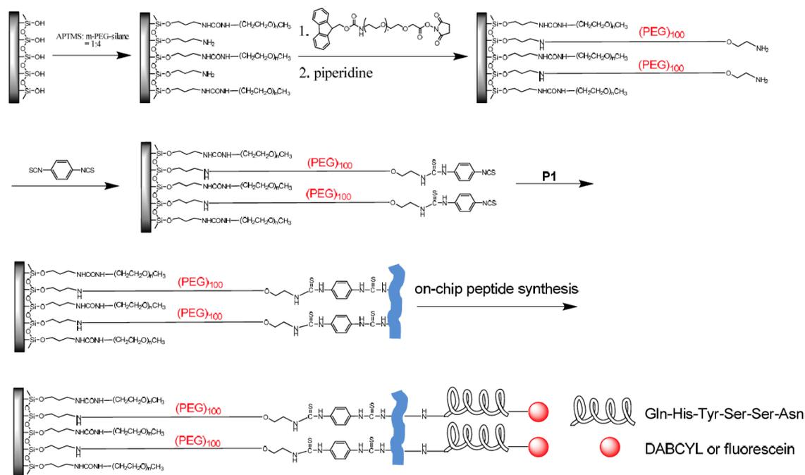
Figure S2. Schematic representation of polymer immobilization onto glass substrate and on-chip peptide synthesis.
