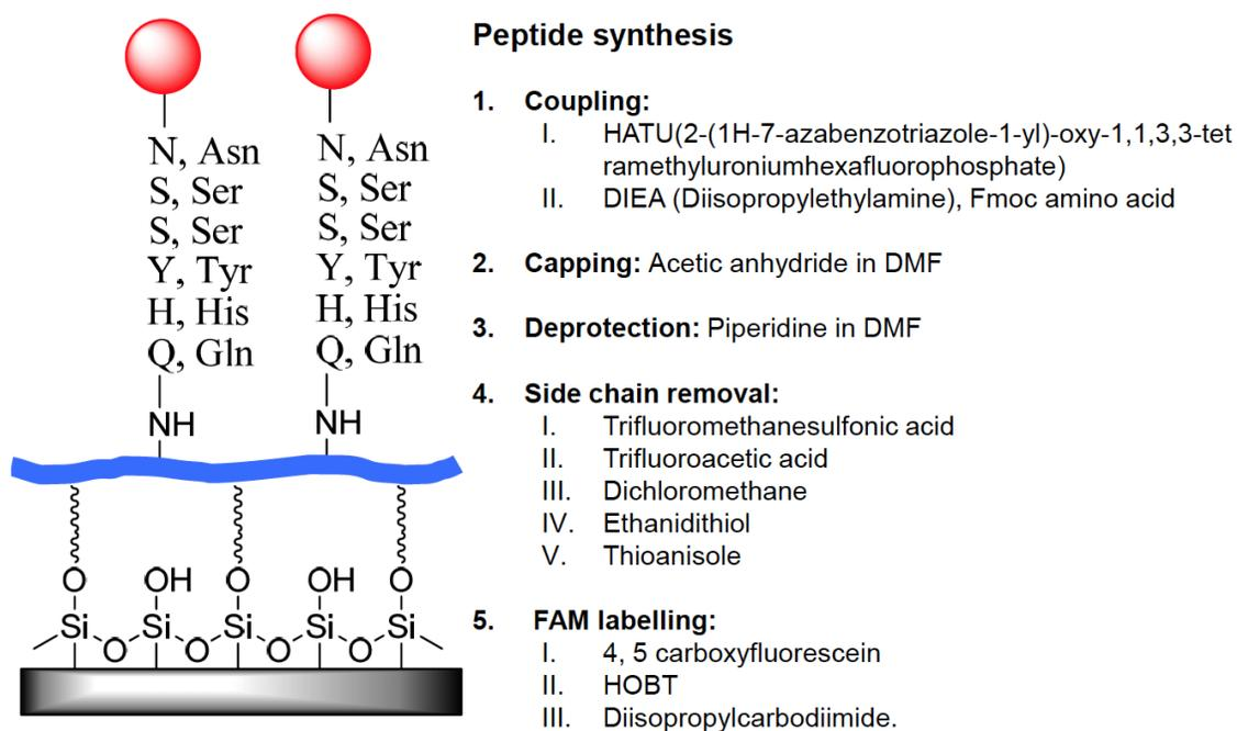
Figure S3. The synthetic procedure of the on-chip peptide synthesis on the P1-coated substrate and the reagents used for the synthesis.
