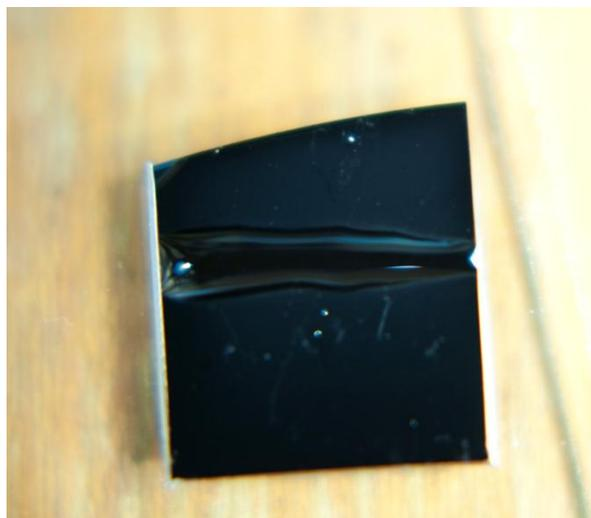
**Fig. S5** Using the APMPJ treatment, a thin strip could be created on the surface of the CNT arrays. This microfluidic strip allowed the control of a small volume of liquid at the microscale with high precision. Shown above is an example of the aqueous solution containing Au nanodots dropped onto the microfluidic strip. It was found that the solution was confined within the plasma-generated microfluidic strip.
