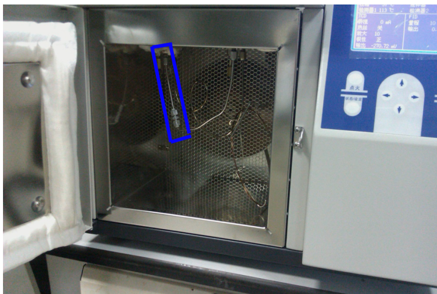
Fig. s10. Optical photo of the interior of the Column Compartment of the GC used in the present work.
