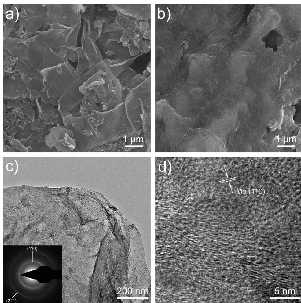
**Figure S10.** a), b) SEM images of as-prepared MoS<sub>2</sub>NS/RGO electrode. b), c), d) SEM, TEM, and HRTEM images of MoS<sub>2</sub>NS/RGO electrode after 700 cycles, the inset in c) shows the corresponding SAED pattern.
