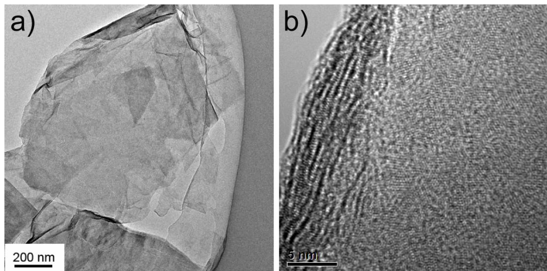
**Figure S6.** a) TEM image and b) HRTEM image of  $\text{MoS}_2$  nanosheets.
