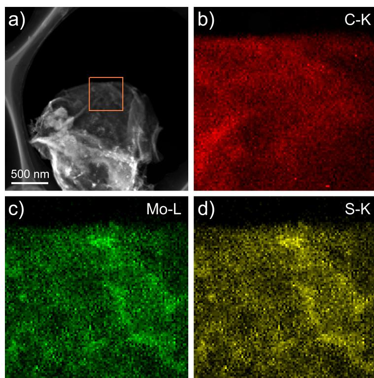
**Figure S11.** a) STEM image, b), c), and d) carbon, molybdenum, and sulfur element mapping images of  $\text{MoS}_2\text{NS/RGO}$  after 700 cycles, respectively.
