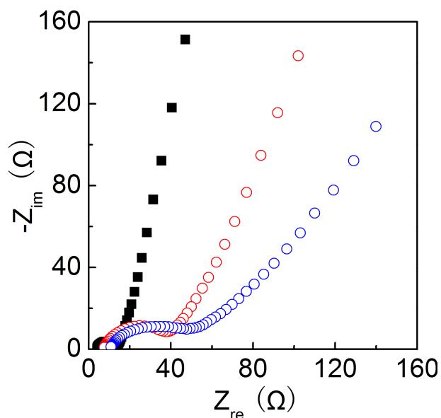
**Figure S9.** Nyquist plots of MoS<sub>2</sub>NS/RGO electrodes before cycling (black squares), after 3 cycles (red circles), and after 700 cycles (blue circles).
