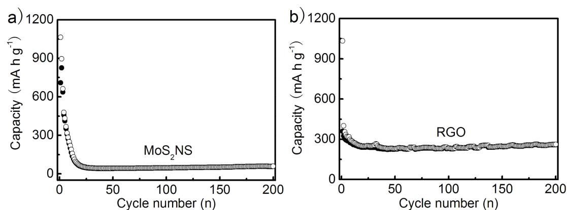
**Figure S8.** Cycling performance of MoS<sub>2</sub>NS electrode and RGO electrode at a current density of 0.5  $\text{A g}^{-1}$  in the voltage range of 0.005–3 V vs Li<sup>+</sup>/Li.
