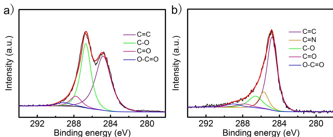
**Figure S4.** XPS C 1s spectra of a) GO and b) MoS<sub>2</sub>NS/RGO. the main peaks centered at 284.8 eV corresponding to extensively delocalized  $\text{sp}^2$ -hybridized carbon atoms, and the independent peaks with binding energies of 285.7, 286.6, 287.8, and 289.0 eV can be attributed to carbon atoms in C=N, C-O, C=O, and O-C=O, respectively.
