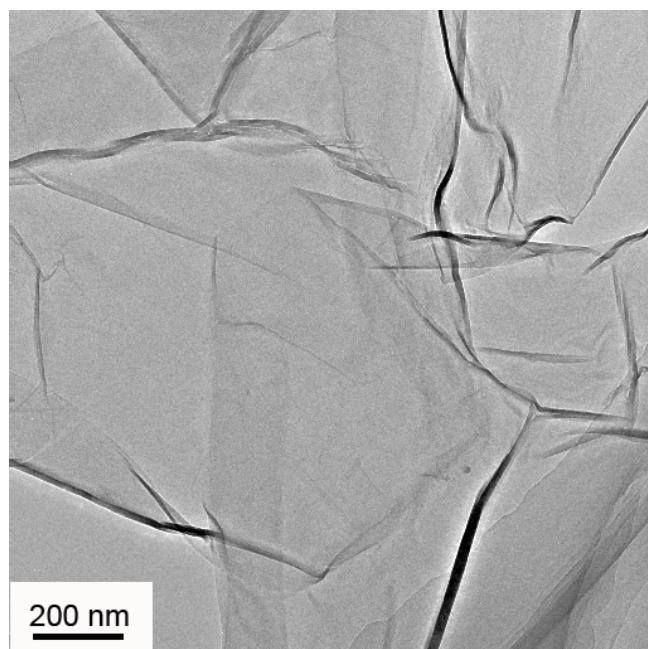
**Figure S7.** TEM image of reduced graphene oxide.
