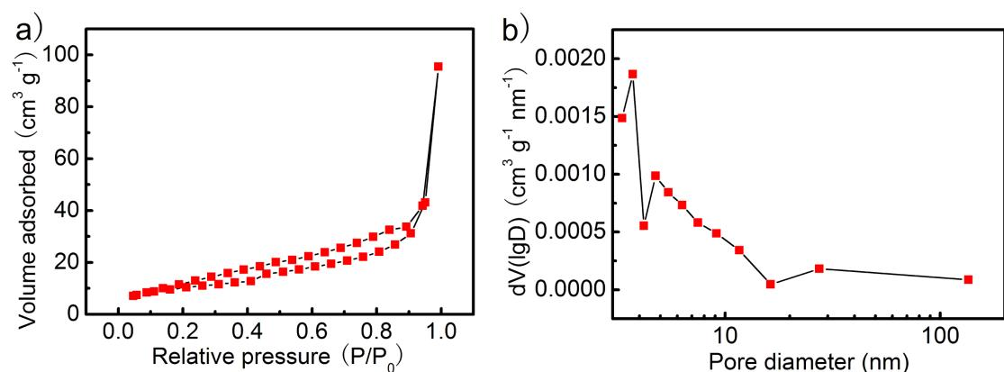
**Figure S5.** a) Nitrogen adsorption/desorption isotherms of  $\text{MoS}_2$  NS/RGO, (b) pore-size distribution plot calculated by the BJH formula with the desorption isotherm.
