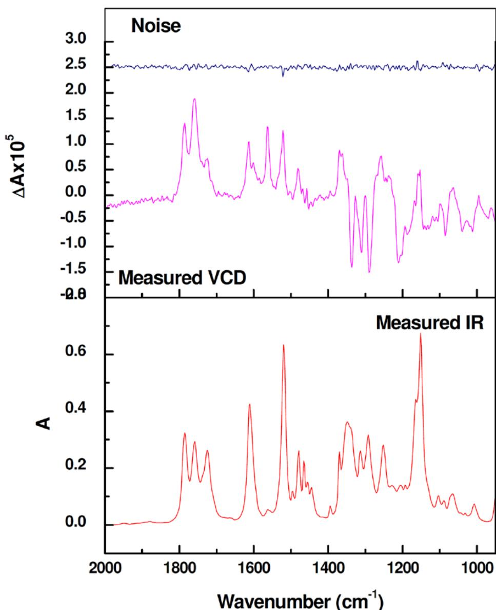
**Figure 1.** IR (lower frame) and VCD (upper frame) spectra of **5a** in  $\text{CDCl}_3$  (5.2 mg/0.15 mL); 100- $\mu\text{m}$  path-length cell with  $\text{BaF}_2$  windows; 23 h collection for sample and solvent; instrument optimized at  $1400\text{ cm}^{-1}$ . Solvent-subtracted spectra are shown. Uppermost trace is the VCD noise.
