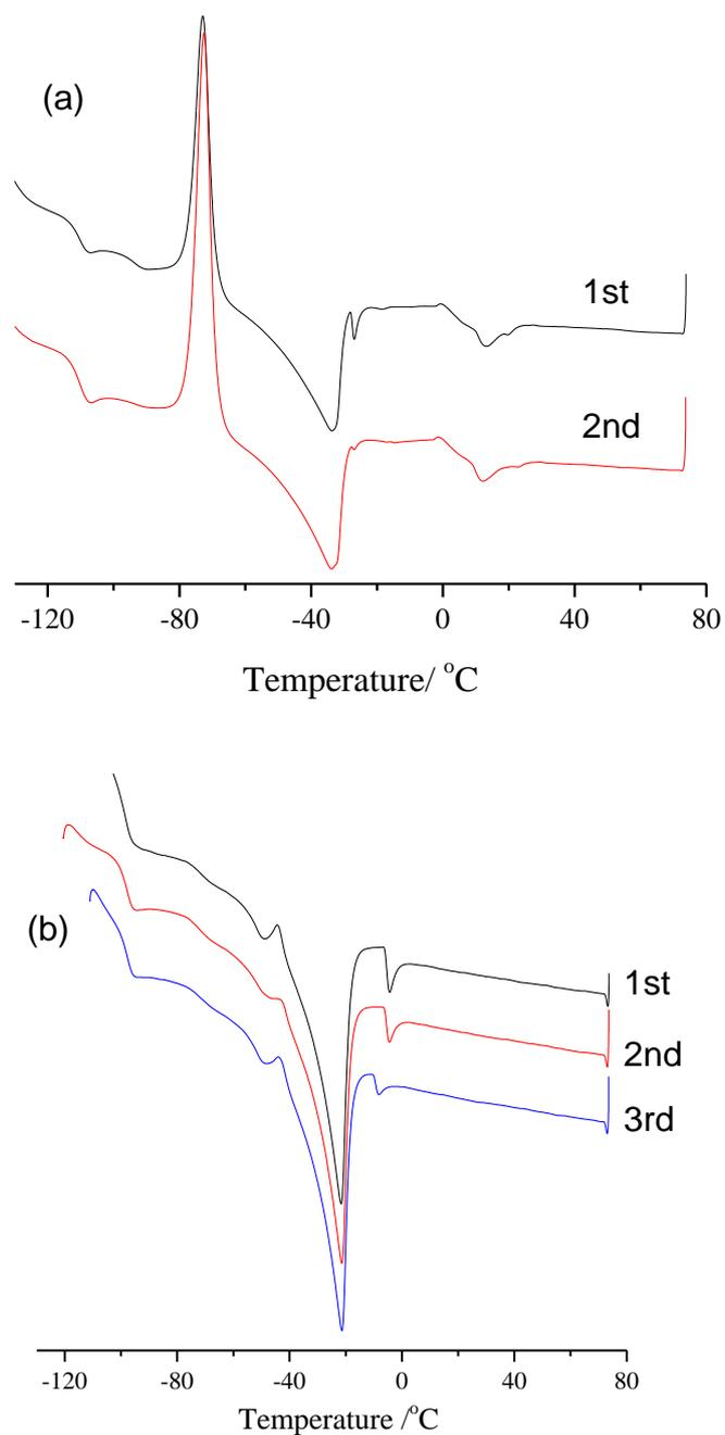
**Figure S1.** Effect of cycle time on DSC charts of Hy[ch][dhp] with water contents of 7:1 (a) and Hy[ch][dBp] with water contents of 12:1 (b).
