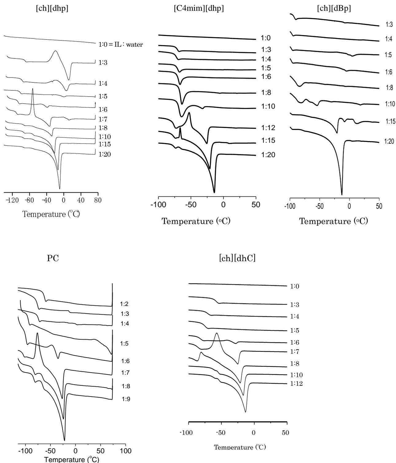
**Figure S2.** DSC heating curves of hydrated ILs with different water content.
