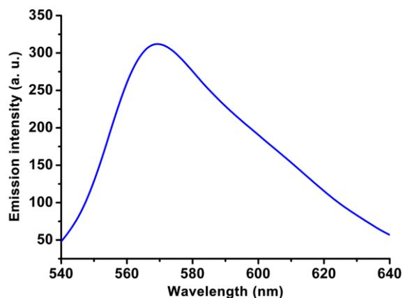
**Fig. S2** Emission spectrum ( $\lambda_{\text{ex}} = 530 \text{ nm}$ ) of CMDP-OTPBA-R6G-SPION in PBS (pH 7.4).
