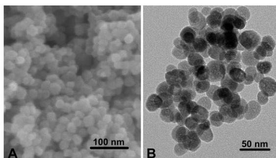
**Fig. S5** SEM (A) and TEM (B) images of  $\gamma$ -Fe<sub>2</sub>O<sub>3</sub> nanoparticles.
