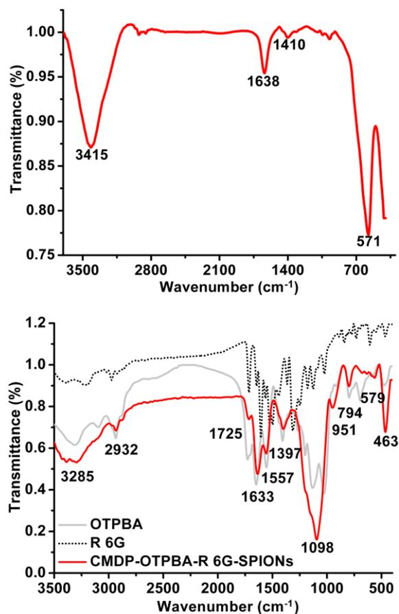
**Fig. S4** FTIR spectra (KBr) of  $\gamma$ -Fe<sub>2</sub>O<sub>3</sub> nanoparticles (top), OTPBA, R6G and CMDP-OTPBA-R6G-SPION (bottom). Attributions (cm<sup>-1</sup>): 3285,  $\nu_{\text{O-H}}$ ; 2932,  $\nu_{\text{CH}_2}$ ; 1725,  $\nu_{\text{C=O}}$  carboxylic acid; 1633,  $\nu_{\text{C=O}}$  amide; 1557,  $\delta_{\text{N-H}}$ ; 1397, 1098,  $\delta_{\text{Si-O}}$ ; 579,  $\nu_{\text{Fe-O}}$ .
