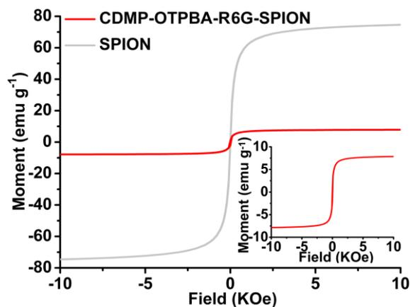
**Fig. S6** Magnetization curve of CMDP-OTPBA-R6G-SPION and SPION at room temperature.
