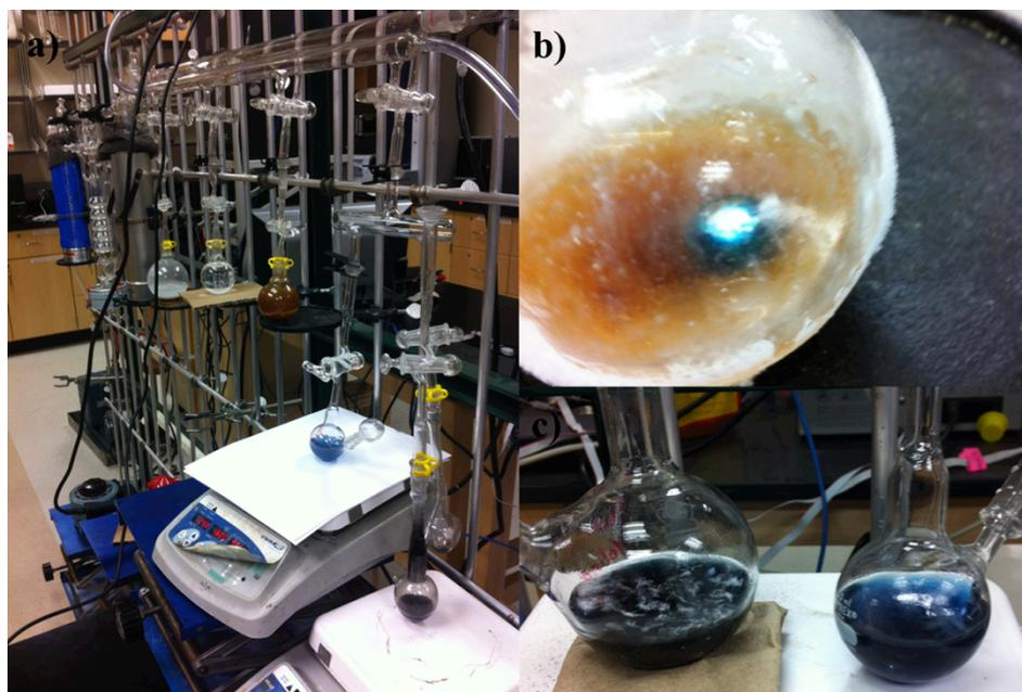
**Figure S1.** (a,b) Vacuum manifold for the purification of 1,2-DME and (c) formation of the deep blue between the Na/K alloy and solvent molecules.
