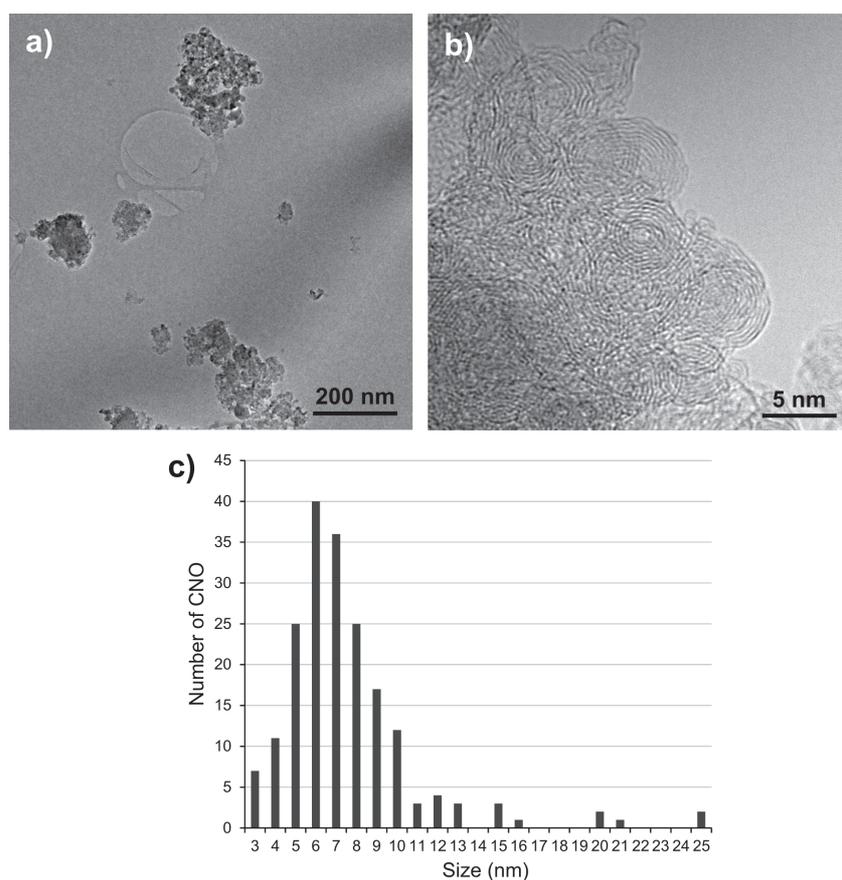
**Figure S5.** TEM images of the Cu holey carbon covered with CNOs-C<sub>16</sub> in NMP/CHCl<sub>3</sub> (1:1, v/v) (a) and (b) after filtration through a 0.1 μm PVDF filter, (c) stadistycal study over 250 TEM pictures.
