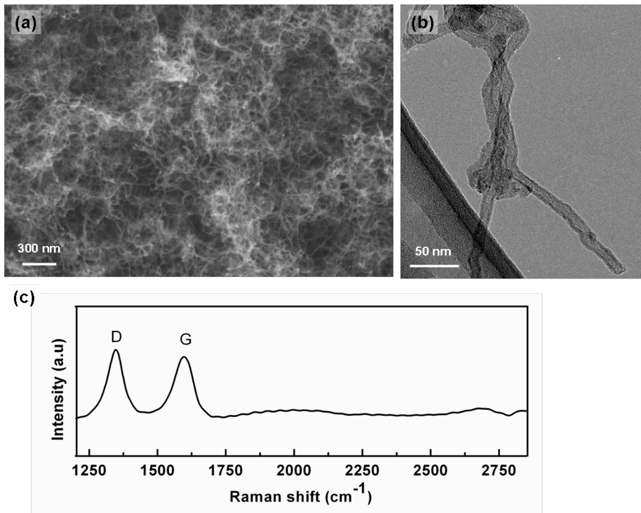
**Figure S3.** Growth of CNTs on SrTiO<sub>3</sub> supported Ni nanocrystals by EtOH-CVD at 700 °C. (a) SEM image of grown sample after the CVD reaction. (b) TEM image of grown CNTs, indicating that there are no particles trapped within the tubes. (c) Representative Raman spectrum confirms the CNT formation on SrTiO<sub>3</sub> substrates.
