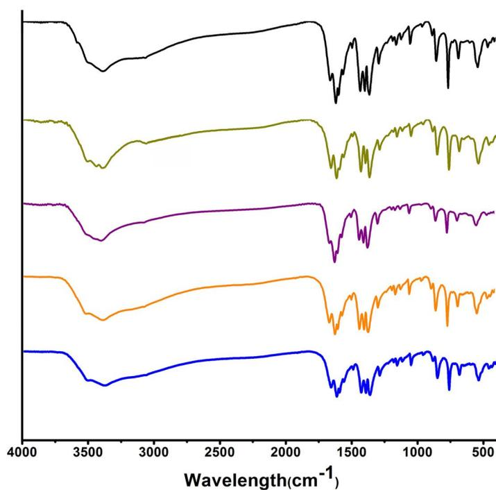
**Fig. S13** FT-IR spectra of as-synthesized **2** (black) and the samples **1** (dark yellow), **2** (purple), **3** (light yellow), **4** (blue) after photocatalytic hydrogen generation.
