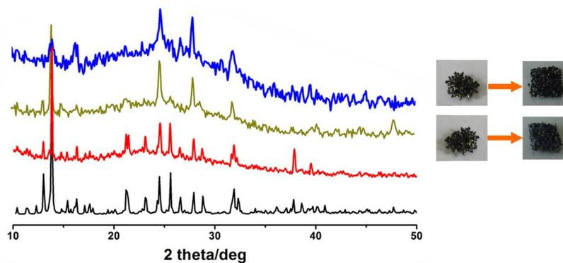
**Fig. S7** XRPD patterns of **2** after soaking in acid (pH = 2, yellow) and base solutions (pH = 12, blue). The photos of the crystals before and after soaking in acid solutions and base solutions are shown in the right side of each spectrum, respectively.
