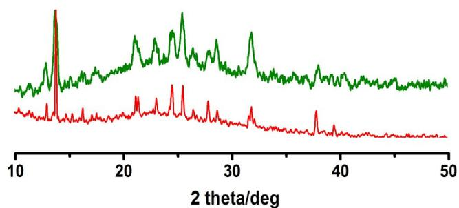
**Fig. S9** XRPD patterns of as-synthesized **2** (red) and after releasing  $I_2$  of **2** (green).
