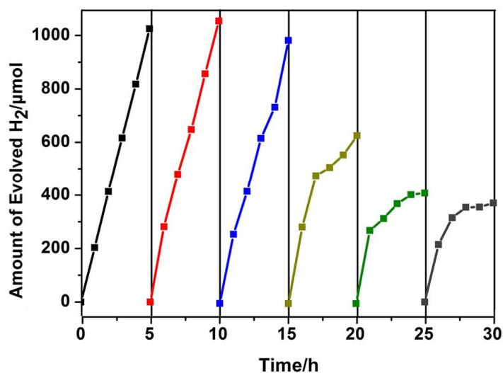
**Fig. S11** Time course of H<sub>2</sub> evolution from compound **3** dissolved in 100 mL of 10% methanol solution under UV irradiation using a 500 W mercury lamp.
