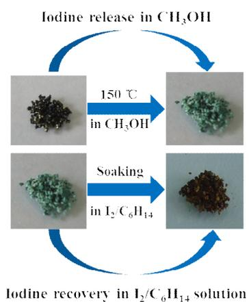
**Fig. S8** The photographs of **2** for releasing  $I_2$  in methanol at 150°C and **2a** for adsorbing  $I_2$  in hexane.
