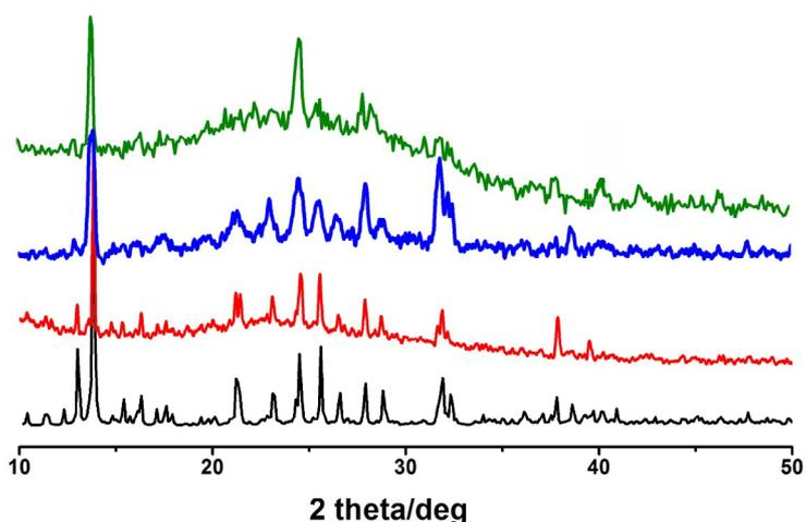
**Fig. S6** XRPD patterns of **2** after treated in boiling water for 3 days (green) and exposed it to air for 3 months (blue).
