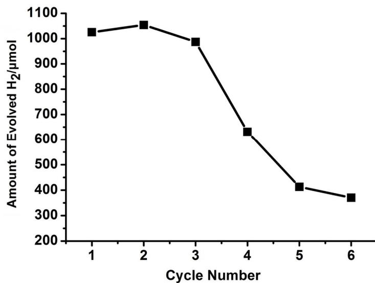
**Fig. S12** The hydrogen evolution cycle property in compound **3**.
