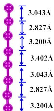
**Fig. S4** The iodine–iodine distances of the repeated unit I(1)–I(2)–I(3)–I(4)–I(5)–I(6)–I(7)–I(8).
