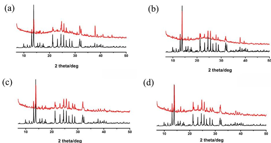
**Fig. S1** X-ray powder diffraction patterns of as-synthesized (red) and simulated (black) **1** (a), **2** (b), **3** (c) and **4** (d).
