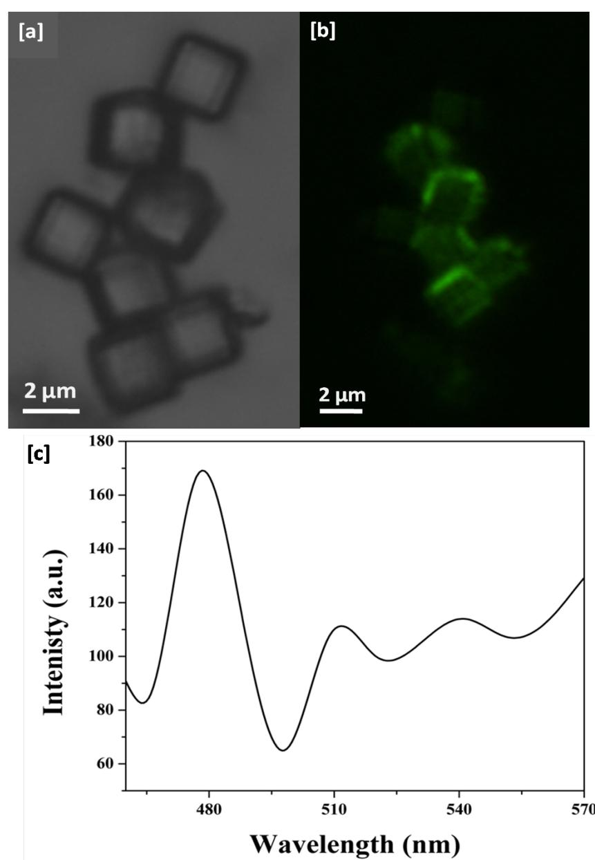
**Fig. S11.** Confocal laser scanning microscopic images (CLSM) of  $[Zn(C_4O_4)(H_2O)_2]$  cubes after functionalization with OPV-NH<sub>2</sub>. cubes (a) without excitation (b) with excitation at 421 nm showing green fluorescent cubes and (c) corresponding emission spectra of the cubes obtained under the confocal microscope.
