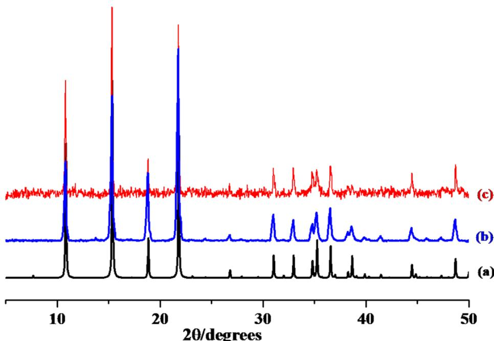
**Fig. S3.** Powder X-ray diffraction (PXRD) pattern of the nanocages. (a) simulated pattern of  $[\text{Co}(\text{C}_4\text{O}_4)(\text{H}_2\text{O})_2]_n$ ; (b) assynthesized nanocage of  $[\text{Zn}(\text{C}_4\text{O}_4)(\text{H}_2\text{O})_2]_n$ ; (c) assynthesized cage of  $[\text{Cd}(\text{C}_4\text{O}_4)(\text{H}_2\text{O})_2]_n$ .
