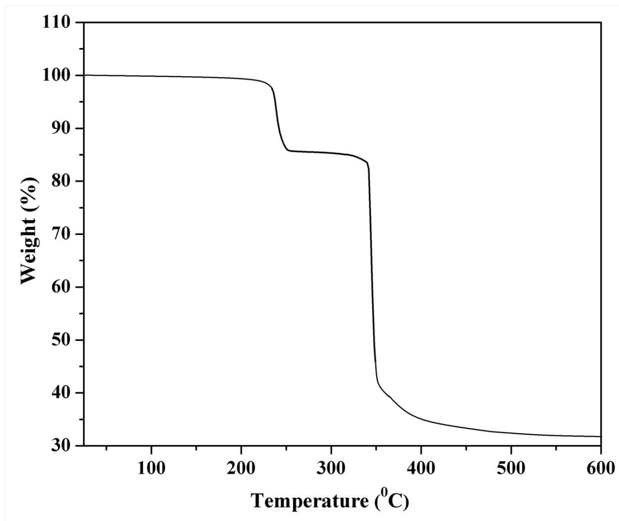
**Fig. S2a.** Thermogravimetric analysis (TGA) of cage of  $[\text{Co}(\text{C}_4\text{O}_4)(\text{H}_2\text{O})_2]$  (**1**).
