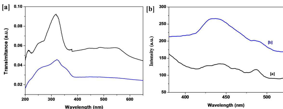
**Fig. S9.** [a] UV-vis spectra and [b] emission spectra of squaric acid and  $[Zn(C_4O_4)(H_2O)_2]_n$  (**2**) cages. (black line for squaric acid and blue line for  $[Zn(C_4O_4)(H_2O)_2]_n$  nanocages)
