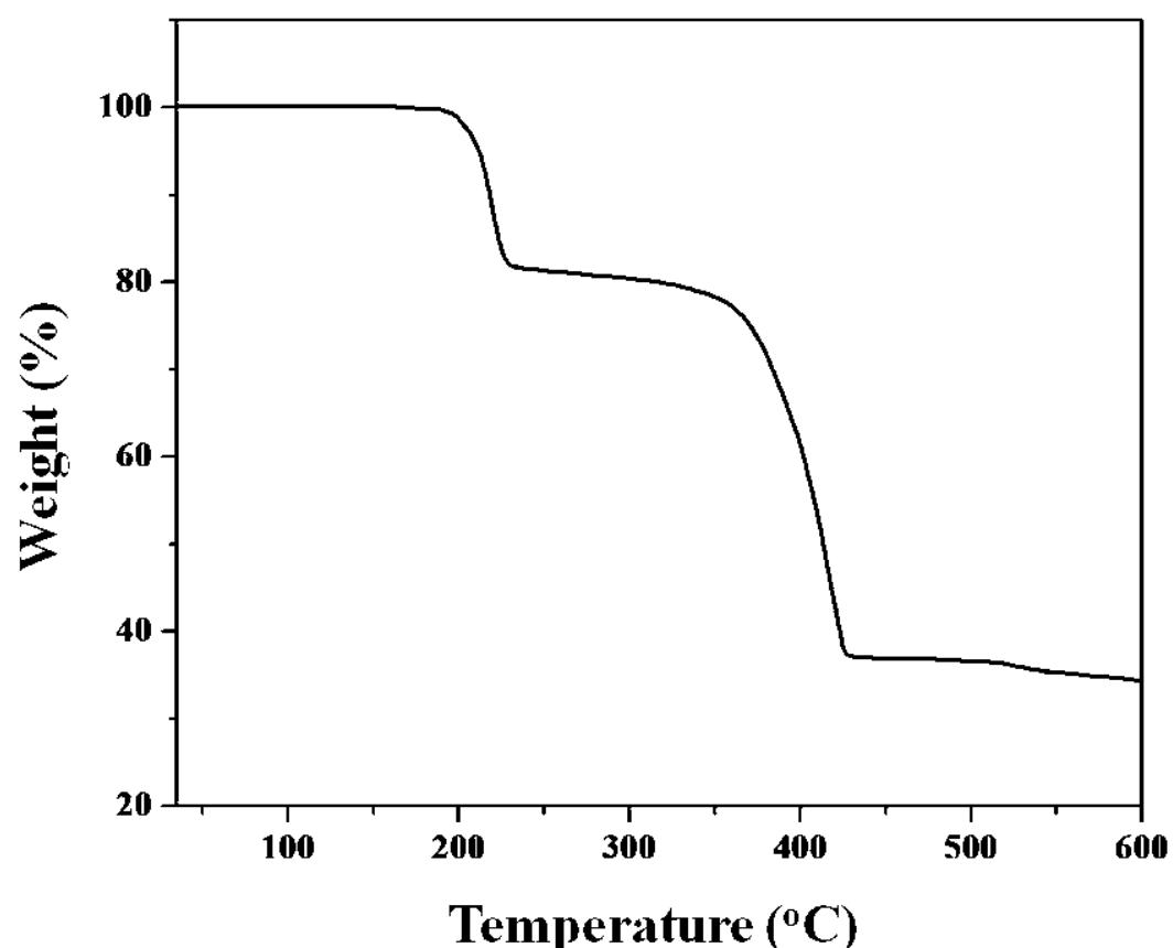
**Fig. S2b.** Thermogravimetric analysis (TGA) of cage of  $[\text{Zn}(\text{C}_4\text{O}_4)(\text{H}_2\text{O})_2]$  (**2**).
