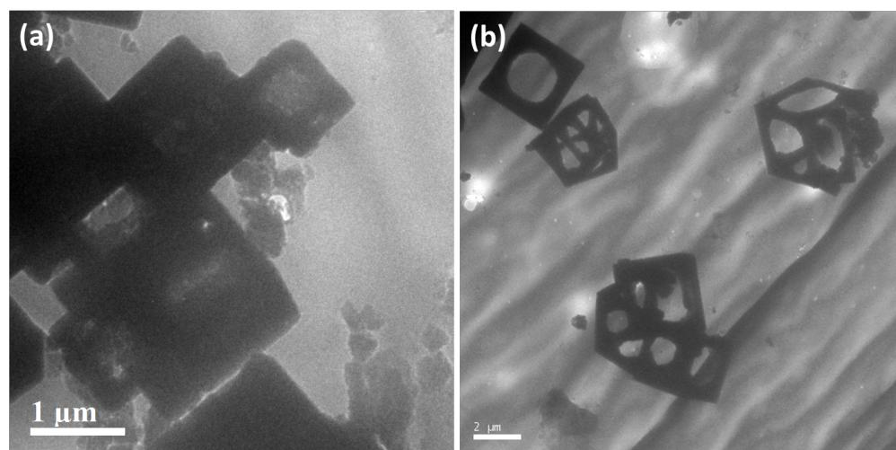
**Fig. S5b.** TEM images of (a)  $[\text{Zn}(\text{C}_4\text{O}_4)(\text{H}_2\text{O})_2]$  (2) ; (b)  $[\text{Cd}(\text{C}_4\text{O}_4)(\text{H}_2\text{O})_2]$  (3) showing micronic cages throughout the sample.
