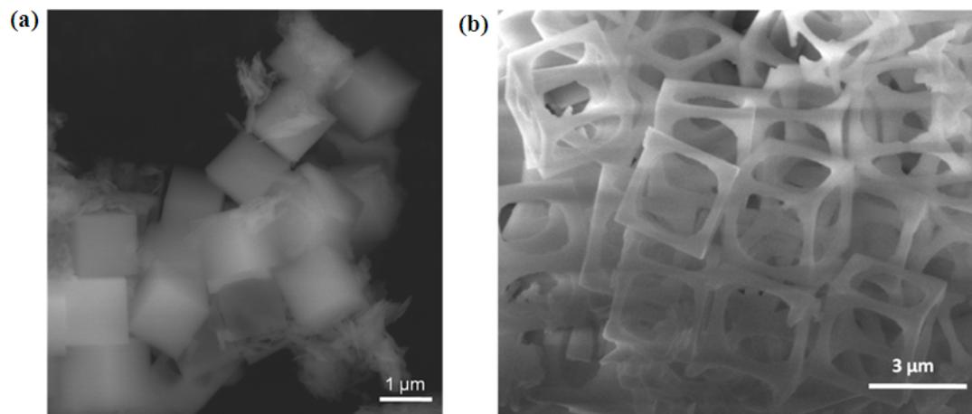
**Fig. S5a.** (a) Cubes of  $[\text{Co}(\text{C}_4\text{O}_4)(\text{H}_2\text{O})_2]$  (1) obtained in good yield after 24 h of reaction time. (b) Cages of  $[\text{Co}(\text{C}_4\text{O}_4)(\text{H}_2\text{O})_2]$  (1) obtained in good yield after 96 h of reaction time.
