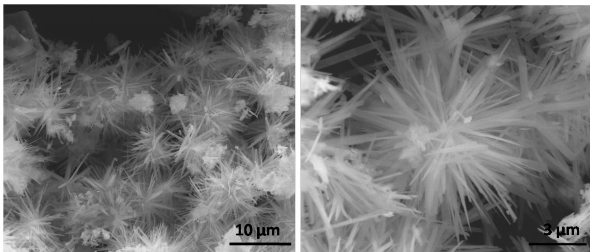
**Fig. S6.** Dandelion-like nanostructures obtained after 24 h reaction time while using lower amount of PVP.
