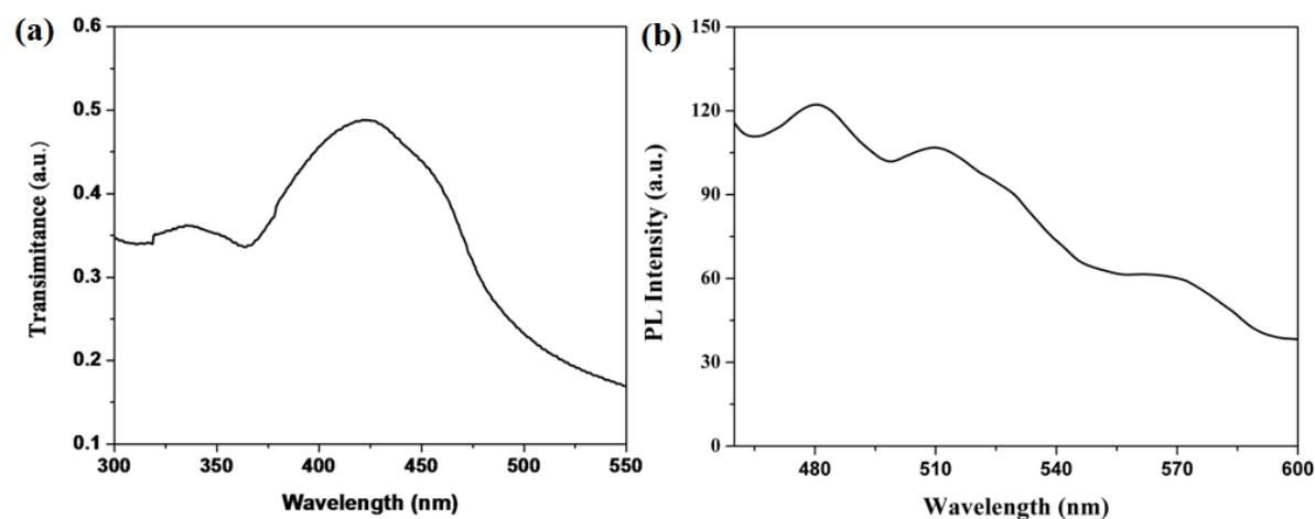
**Fig. S10.** (a) UV-vis and (b) emission spectra of OPV-NH<sub>2</sub> in solid state.
