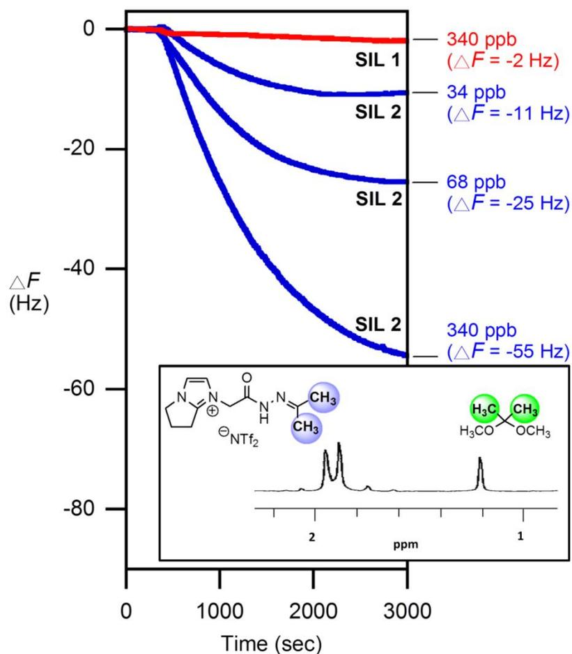
**Fig. S4** Sensitive detection of 2,2-dimethoxypropane gas, a masked acetone, by 9 MHz QCM thin-coated with **SIL 2** (3.3 nL each, 300 nm thickness) containing 2 mol%  $\text{Sc}(\text{OTf})_3$ . Gas samples were injected at 300 s. The resonance frequency drop,  $\Delta F$ , is the QCM response on the quartz chip surface. Inset:  $^1\text{H}$  NMR detail of the conversion confirmation of the imine forming reaction.
