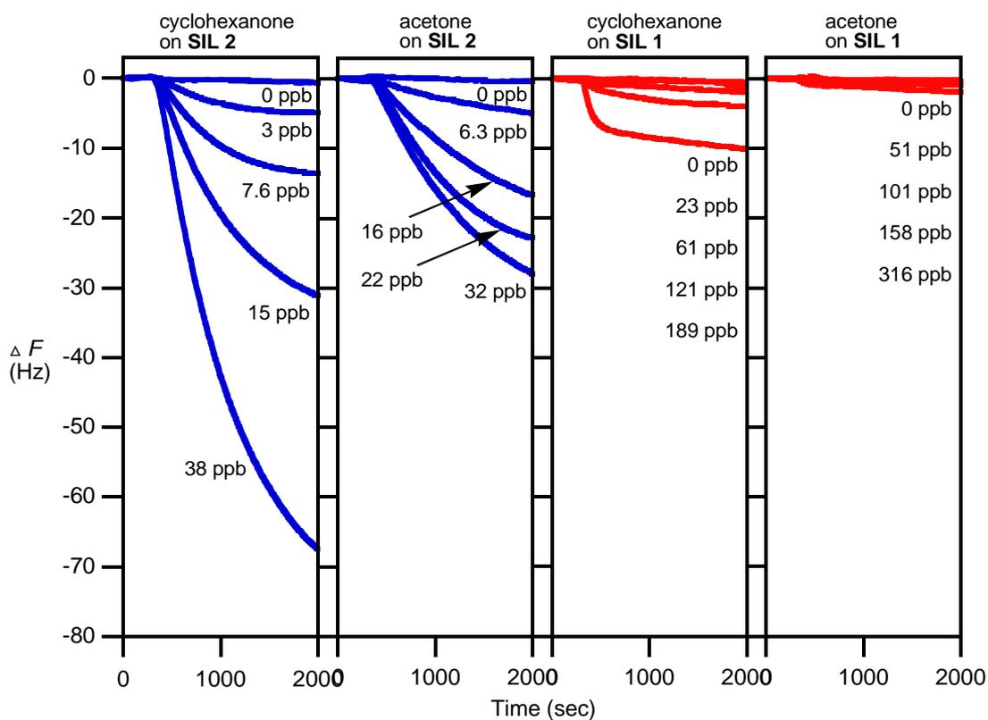
**Fig. S3** Sensitivity detection of acetone and cyclohexanone gases using 9 MHz QCM thin-coated with **SIL 1** and **SIL 2** (3.3 nL each, 300 nm thickness) containing 2 mol%  $\text{Sc}(\text{OTf})_3$ . Ketone gas samples were injected at 300 s. The resonance frequency drop,  $\Delta F$ , is the QCM response on the quartz chip surface.
