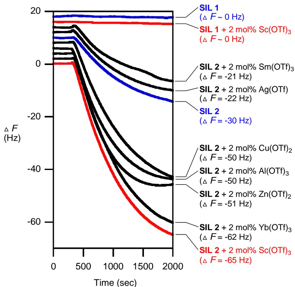
**Fig. S2** Ultrasensitive, Lewis acid-catalyzed detection of acetone gas (58 ppb) by 9 MHz QCM thin-coated with **SIL 1** and **SIL 2** (3.3 nL each, 300 nm thickness) containing various metal triflates (2 mol%). The QCM response curves were vertically shifted (2 Hz in between) for clarity. Gas samples were injected at 300 s. The resonance frequency drop,  $\Delta F$ , is the QCM response on the quartz chip surface.
