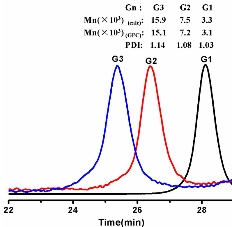
Fig. S22 Molecular weight progress of G1-G3 measured by GPC.
