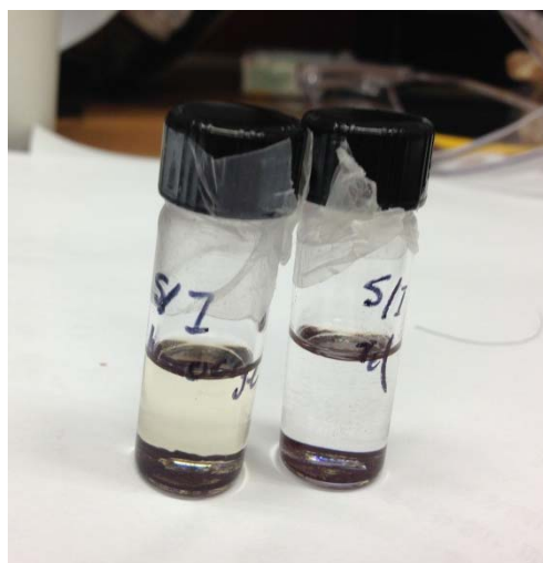
Fig. S11 Left: A toluene solution containing ~0.7 mM of VI with hydrolyzed silyl ester bonds in the presence of \text{PdCl}_2 solid. The yellow color indicated incorporation of Pd ion into VI . Right: Control, a toluene solution containing \text{PdCl}_2 solid.
