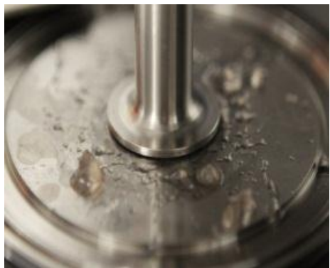
Figure S15: image of a destroyed anhydrous gel ejected due to high shear ( \gamma_0^{\max}=1000\% ).
