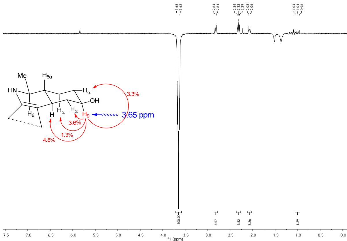
**Figure S13** NOE values observed by irradiation of H-9, the remaining part of the molecule was omitted for clarity.
