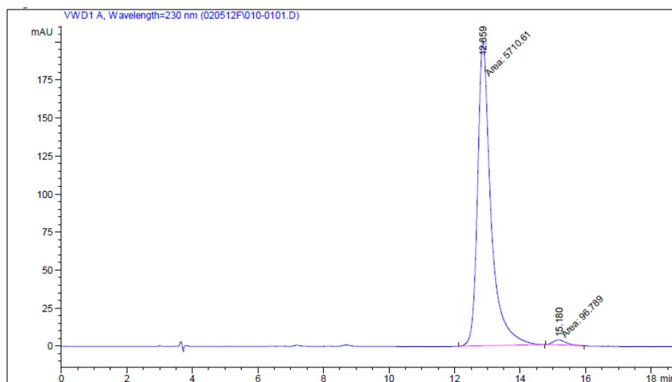
**Figure S7** Chiral HPLC chromatogram of **9** (97% *ee*, prepared from optically pure **2** and (*S*)-**5** with 97% *ee*)
