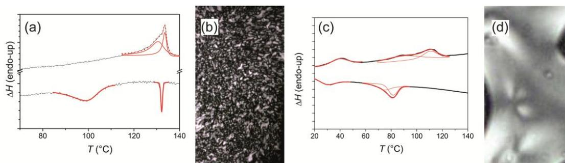
**Figure S1:** (a) DSC of compound **2** at 2 K min<sup>-1</sup> and (b) polarized optical microscopy image of **2** at 20 °C. The birefringent phase proves the presence of a liquid-crystalline phase at room temperature. (c) DSC of compound **4** at 2 K min<sup>-1</sup> and (d) POM image of **4** at 40 °C after melting, indicating a liquid-crystalline phase.
