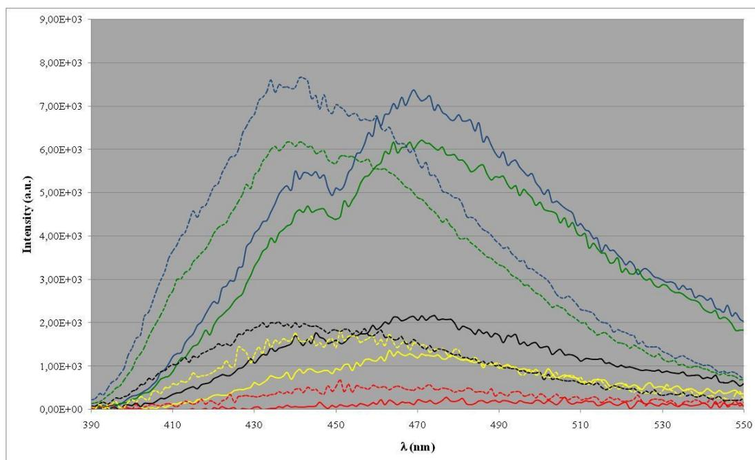
**Figure S3:** Emission spectra of **2**,  $3.03 \times 10^{-5}$  M (black),  $9.08 \times 10^{-4}$  M (blue),  $4.54 \times 10^{-4}$  M (green),  $2.27 \times 10^{-3}$  M (yellow), Gel  $20 \text{ mg mL}^{-1}$  (red), and **4**,  $3.15 \times 10^{-5}$  M (dashed black),  $8.90 \times 10^{-4}$  M (dashed blue),  $4.11 \times 10^{-4}$  M (dashed green),  $1.98 \times 10^{-3}$  M (dashed yellow), Gel  $20 \text{ mg mL}^{-1}$  (dashed red).
