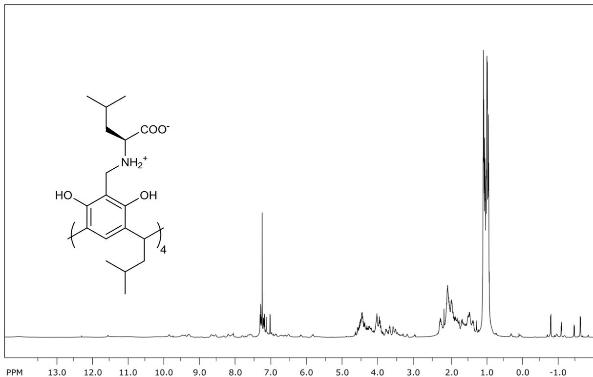
Figure 3. <sup>1</sup>H NMR spectrum of (L-2c)<sub>2</sub>
