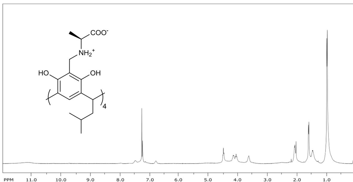
Figure 1. <sup>1</sup>H NMR spectrum of (L-2b)<sub>2</sub>
