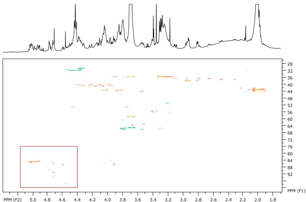
Figure 12. HSQC spectrum of a reaction mixture after 1 day (CDCl<sub>3</sub>, 298 K, 600 MHz).
