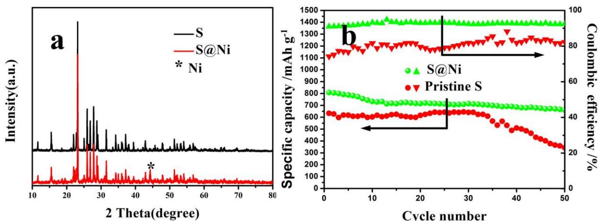
**Fig. S6.** (a) XRD pattern of Ni@S and pristine S. (b) Cycling performance of S and Ni@S at a current density of 0.1 C.
