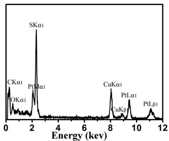
Fig. S3. EDX of Pt@S particle
