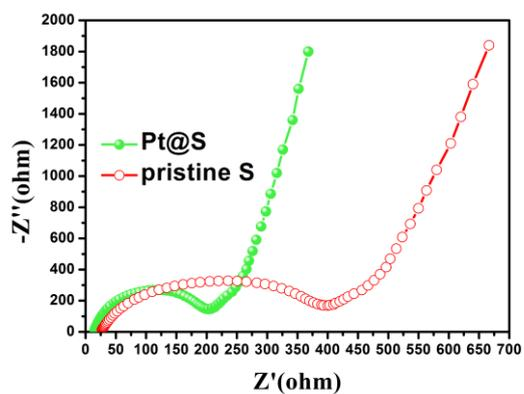
Fig. S4. EIS spectra of pristine S electrodes and Pt@S electrodes
