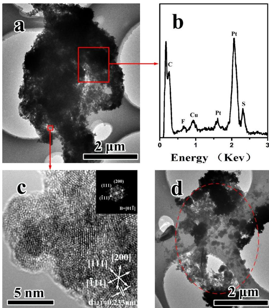
**Fig. S5.** (a) TEM image of Pt@S particle after 50 cycling. (b) EDX of (a). (c) HRTEM image of Pt nanostructures. (d) TEM image of Pt@S particle after 3h heat treatment at 300 °C.
