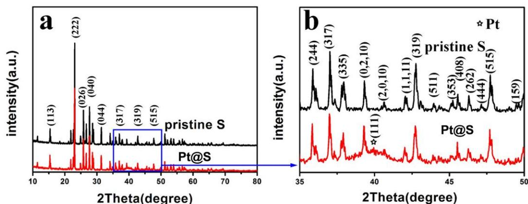
**Fig. S1.** (a) XRD patterns of the Pt@S and the pristine S samples. (b) The partial enlargement of the XRD pattern with 2 theta ranging from 35 to 50 degree.
