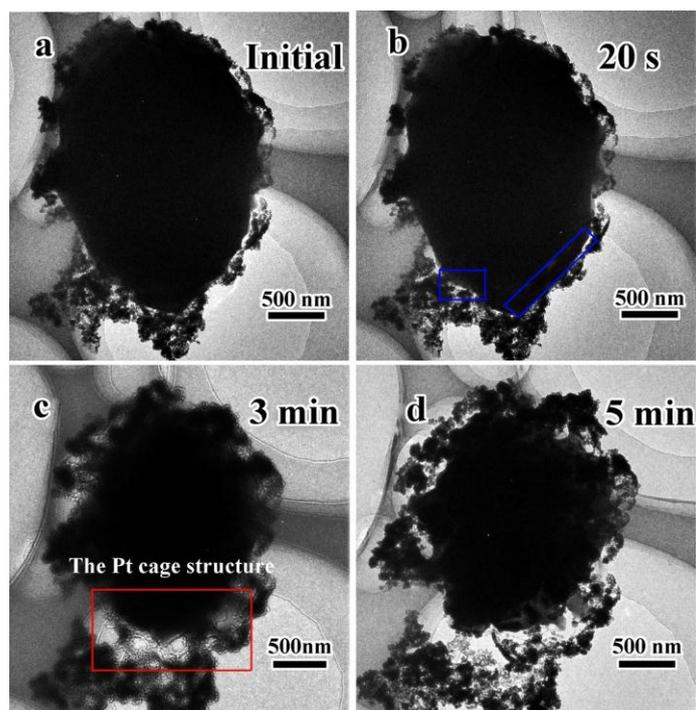
Fig. S2. TEM images of the Pt@S under the electron beam radiation (300KeV)
