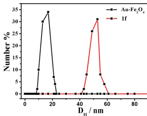
**Fig S3.** Hydrodynamic diameters measured by DLS for the as-synthesized Au-Fe<sub>3</sub>O<sub>4</sub> NPs dispersed in hexane and the **1f** dispersed in PBS.
