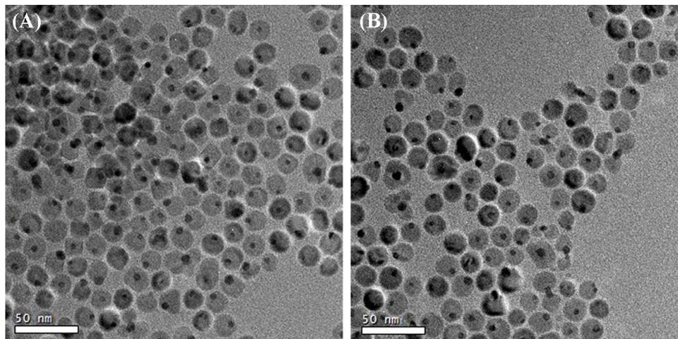
**Fig S1.** TEM images of (A) as-synthesized Au-Fe<sub>3</sub>O<sub>4</sub> nanoparticles dispersed in hexane; (B) **1f** dispersed in H<sub>2</sub>O.
