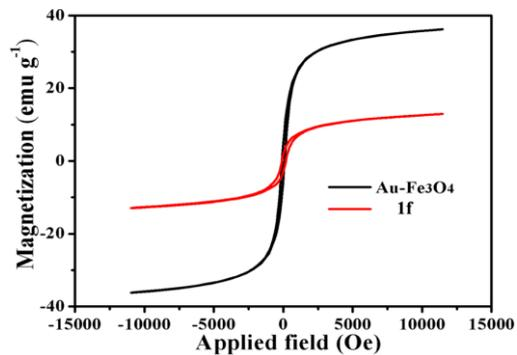
**Fig S2.** Magnetization measured at 300 K. The saturated magnetization ( $M_s$ ) of as-synthesized Au-Fe<sub>3</sub>O<sub>4</sub> Nps and **1f** are 36.2 and 17.6 emu/g.
