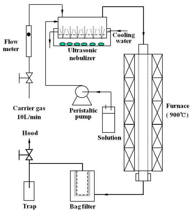
**Fig. S1** Schematic diagram of the ultrasonic spray pyrolysis process.
