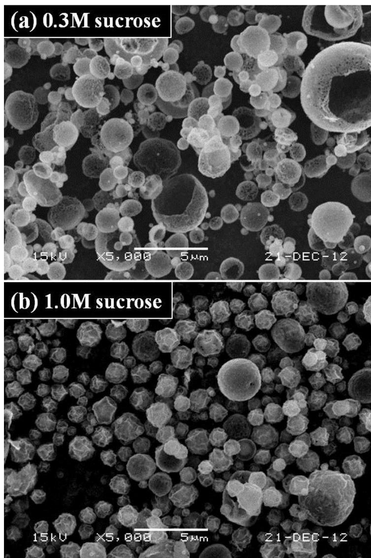
**Fig. S5** SEM images of the  $\text{Co}_3\text{O}_4$  powders prepared by spray pyrolysis at  $900^\circ\text{C}$  from the spray solutions with various concentrations of sucrose.
