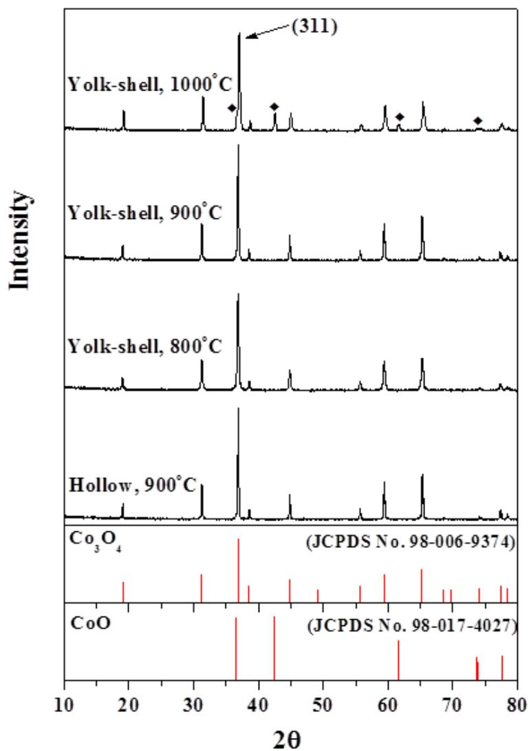
**Fig. S4** XRD patterns of the yolk-shell and hollow Co<sub>3</sub>O<sub>4</sub> powders prepared by spray pyrolysis from the spray solutions with and without sucrose.
