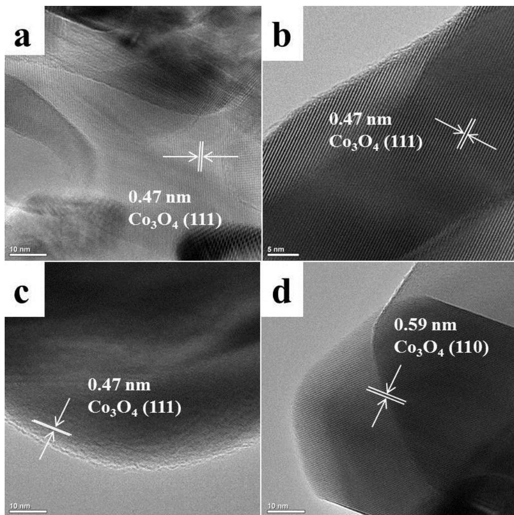
**Fig. S2** HR-TEM images of the  $\text{Co}_3\text{O}_4$  powders; (a) yolk-shell, 800°C, (b) yolk-shell, 900°C, (c) yolk-shell, 1000°C, (d) hollow, 900°C.
