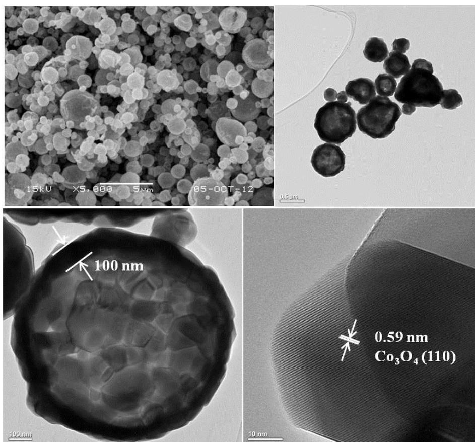
**Fig. S3** SEM and TEM images of the hollow  $\text{Co}_3\text{O}_4$  powders prepared by spray pyrolysis from the spray solution without sucrose at  $900^\circ\text{C}$ .
