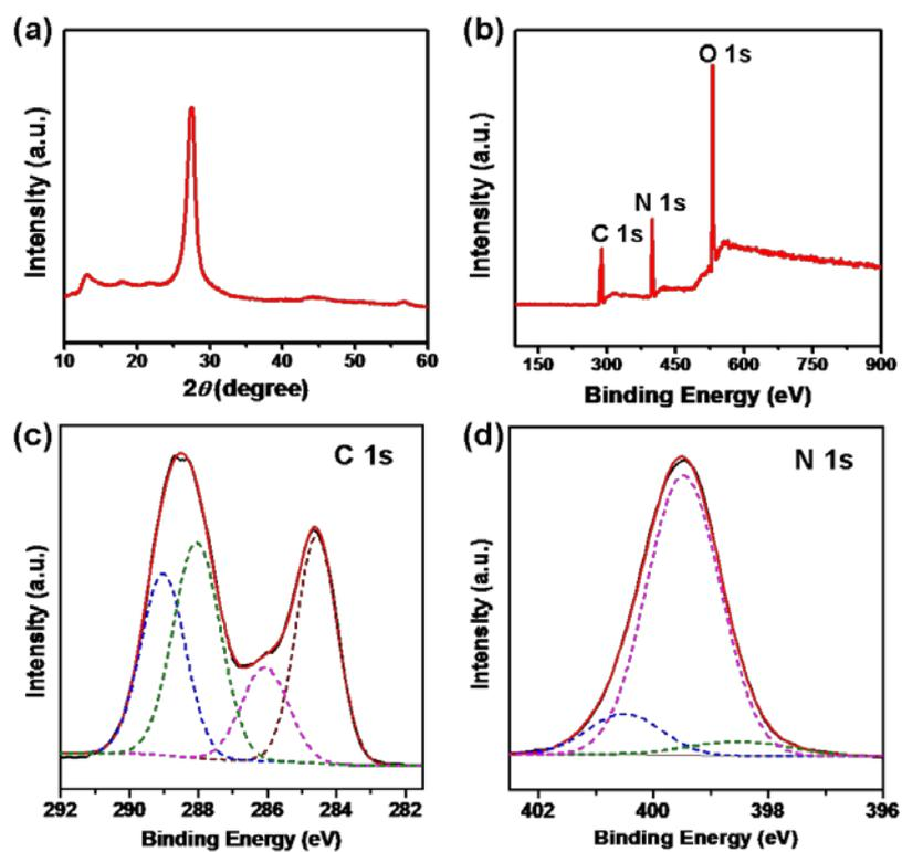
**Fig. S1** (a) XRD spectra and (b) XPS spectra of the obtained g-CNQDs. (c) and (d) are the corresponding C1s spectrum and N1s spectrum of g-CNQDs.
