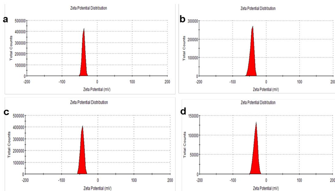
**Fig. S3** Average zeta potential of the obtained carbon nitride dots. (a) -38.5 mV, urea and sodium citrate with the molar ratio of 3:1; (b) -42.4 mV, urea and sodium citrate with the molar ratio of 6:1; (c) -42.5 mV, urea and sodium citrate with the molar ratio of 9:1; (d) -31.6 mV, urea and sodium citrate with the molar ratio of 12:1.
