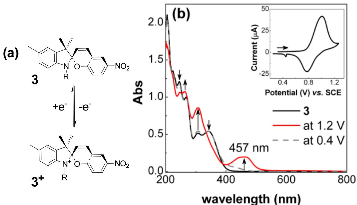
**Fig. S6** (a) Reversible oxidation of methyl-nitro-spiropyran **3**. R = -C<sub>2</sub>H<sub>4</sub>-OC(=O)-C<sub>7</sub>H<sub>15</sub>. (b) UV/vis absorption spectra of **3** recorded upon oxidation in acetonitrile (0.1 M TBAPF<sub>6</sub>) at a scan rate 0.05 V s<sup>-1</sup>. Upon reduction **3** is recovered. Partial photochemical conversion to the MC form occurs during spectra acquisition, manifested in the absorption at *ca.* 430 nm.
