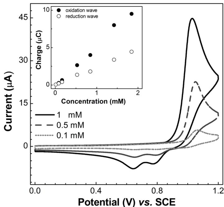
**Fig. S8** Concentration dependent cyclic voltammetry of **1** measured in CH<sub>3</sub>CN (0.1 M TBAPF<sub>6</sub>) at GCE at 0.2 V s<sup>-1</sup>. The charge transferred during the oxidation at 1 V is roughly twice that transferred in the two reduction steps, which is consistent with an initial one-electron oxidation of two spiropyrans (-2e<sup>-</sup>), dimerization and deprotonation to yield a neutral dimer and immediate
