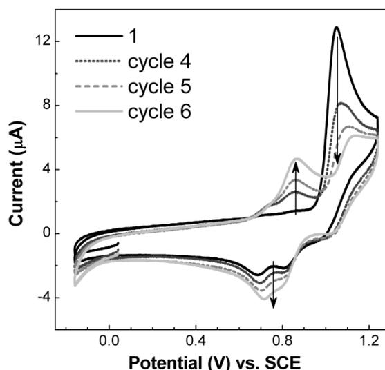
**Fig. S2** Cyclic voltammetry of **1** initially and after few (4-6) cycles of electrolysis measured at glassy carbon electrode vs. SCE in the electrolysis cell in acetonitrile (0.1 M NaClO<sub>4</sub>). Scan rate 0.1 V s<sup>-1</sup>.
