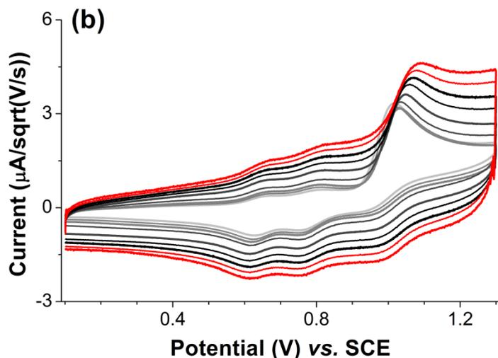
**Fig. S7** Scan-rate dependent cyclic voltammetry of **1** measured in CH<sub>3</sub>CN (0.1 M TBAPF<sub>6</sub>) at GCE at 0.05 V s<sup>-1</sup> – 36 V s<sup>-1</sup>. First (a) and the second (b) cycles of CV show linear dependence of initial oxidation current at *ca.* 1 V on sqrt of scan-rate, plotted in the inset.
