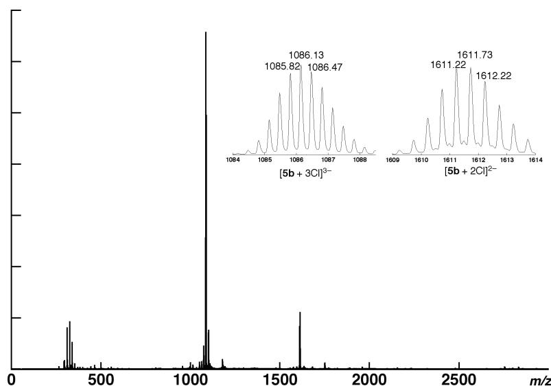
**Supporting Figure 20** ESI-TOF-MS at the negative mode of **5b** with 3.0 equiv of  $\text{Cl}^-$  as a TBA salt from  $\text{CH}_3\text{CN}$  solution ( $1.0 \times 10^{-5} \text{ M}$ ).
