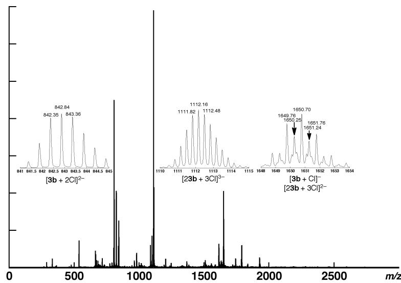
**Supporting Figure 12** ESI-TOF-MS at the negative mode of  $\mathbf{3b}$  with 1.5 equiv of  $\text{Cl}^-$  as a TBA salt from  $\text{CH}_3\text{CN}$  solution ( $1.0 \times 10^{-5} \text{ M}$ ).
