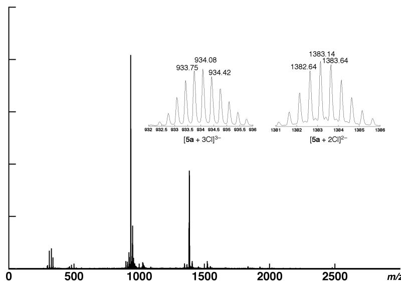
**Supporting Figure 16** ESI-TOF-MS at negative mode of **5a** with 3.0 equiv of  $\text{Cl}^-$  as a TBA salt from  $\text{CH}_3\text{CN}$  solution ( $1.0 \times 10^{-5}$  M).
