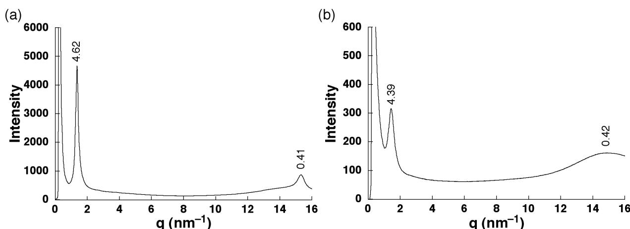
**Supporting Figure 24** XRD patterns of (a) the precipitates of **5c** at r.t. obtained from  $\text{CH}_2\text{Cl}_2/\text{MeOH}$  by drying at r.t. and (b) at r.t. (1st rapid cooling). The measurements were conducted to the dried precipitates in quartz capillary prepared from  $\text{CH}_2\text{Cl}_2/\text{MeOH}$ .
