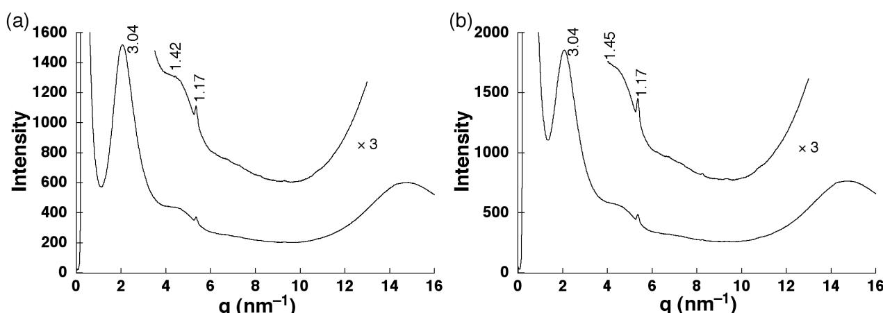
**Supporting Figure 23** XRD patterns of the precipitates of **3c** (a  $\text{Cl}^-$  complex as a  $\text{TATA}^+$  salt) (a) at r.t. obtained from octane (**3c**: 20 mg/mL with 3 equiv of salt) by drying at r.t. and (b) at r.t. (1st rapid cooling). The measurements were conducted to the dried precipitates in quartz capillary prepared from octane solution at r.t. Broad peaks suggest the formation of fairly less ordered packing of **3c** (a  $\text{Cl}^-$  complex as a  $\text{TATA}^+$  salt).
