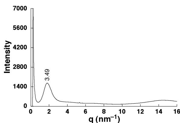
**Supporting Figure 25** XRD patterns of the precipitates of **7c** (a  $\text{Cl}^-$  complex as a  $\text{TATA}^+$  salt) at r.t. obtained from octane (**5c**: 20 mg/mL with 6 equiv of salt) by drying at r.t. The measurements were conducted to the dried precipitates in quartz capillary prepared from octane solution at r.t. Broad peaks suggest the formation of fairly less ordered packing of **5c** (a  $\text{Cl}^-$  complex as a  $\text{TATA}^+$  salt)
