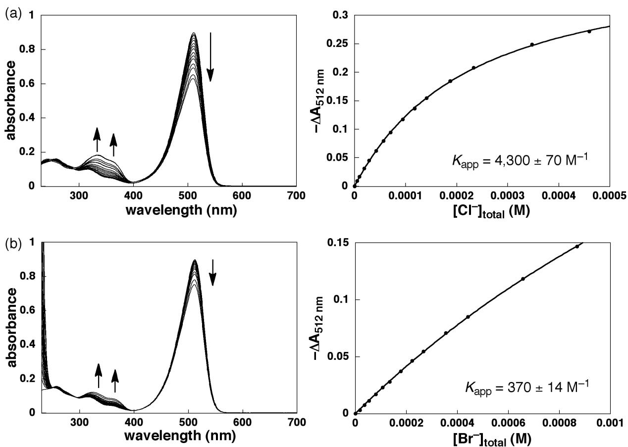
**Supporting Figure 11** UV-vis absorption spectral changes (left) and corresponding titration plots and 1:1 binding fitting curves (right) of  $\mathbf{3b}$  ( $3.0 \times 10^{-6} \text{ M}$ ) upon the addition of (a)  $\text{Cl}^-$  and (b)  $\text{Br}^-$  as TBA salts in  $\text{CH}_2\text{Cl}_2$ .
