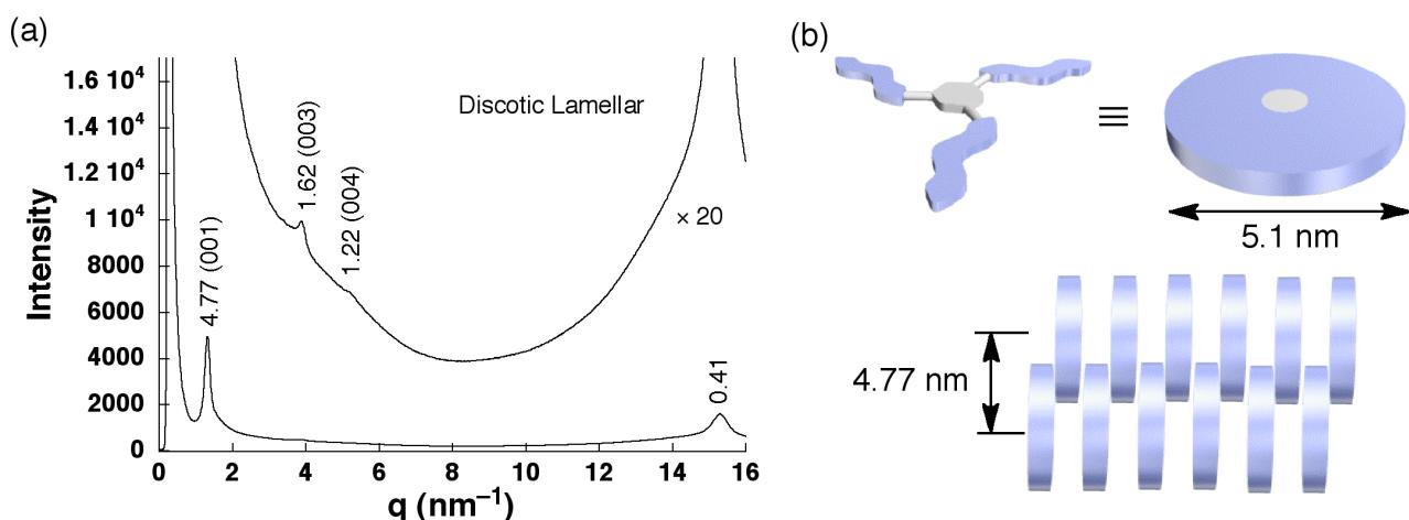
**Supporting Figure 22** (a) XRD patterns of the precipitates of **3c** obtained from CH<sub>2</sub>Cl<sub>2</sub>/MeOH by drying at r.t., and (b) a possible packing structure of **3c**. The measurements were conducted to the dried precipitates in quartz capillary prepared from CH<sub>2</sub>Cl<sub>2</sub>/MeOH.
