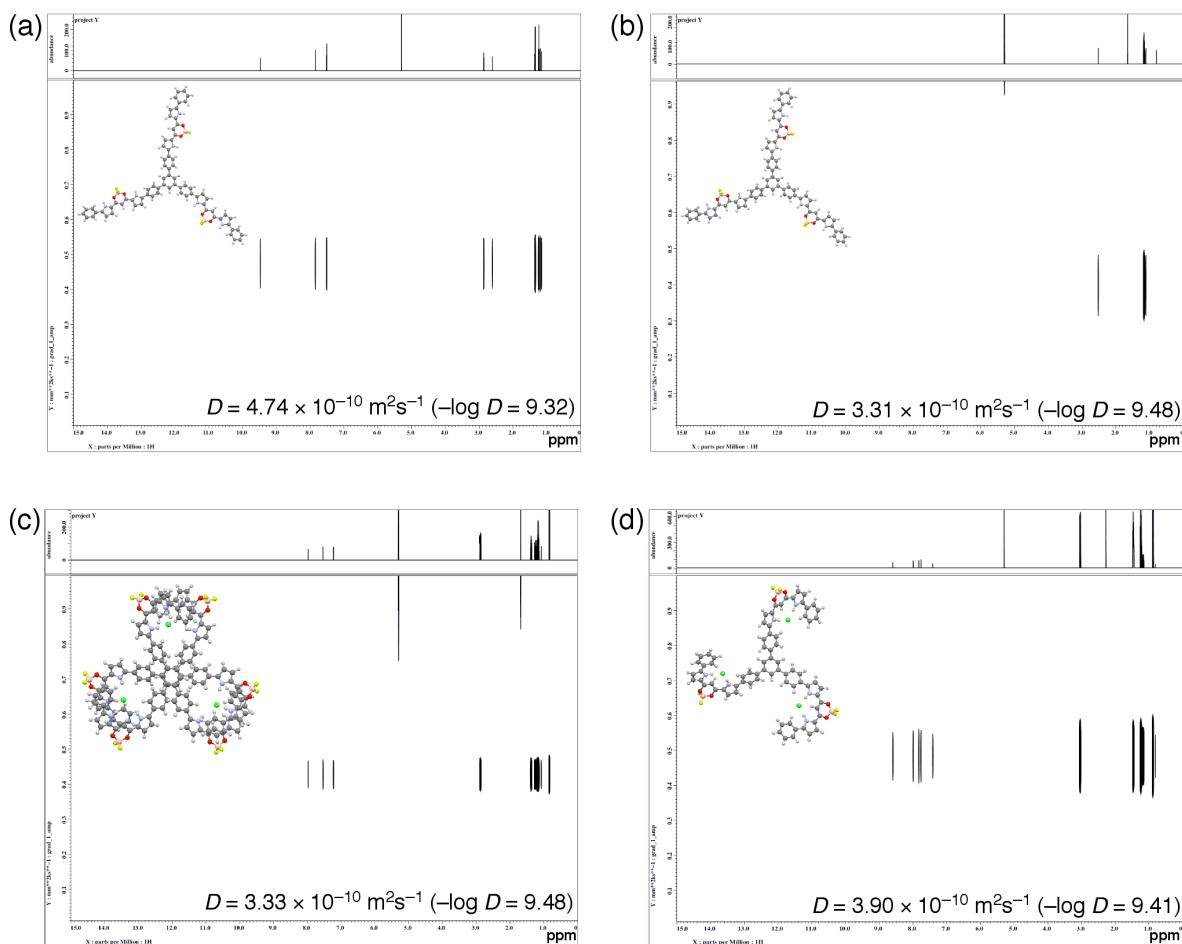
**Supporting Figure 10** <sup>1</sup>H DOSY of **3b** with (a) 0 (at r.t.), (b) 0, (c) 1.5, and (d) 6.0 equiv of Cl<sup>-</sup> added as a TBA salt in CD<sub>2</sub>Cl<sub>2</sub> (1.0 × 10<sup>-3</sup> M) at -50 °C. The smaller *D* value in the absence of TBACl at -50 °C is ascribable to the formation of assemblies of **3b**.
