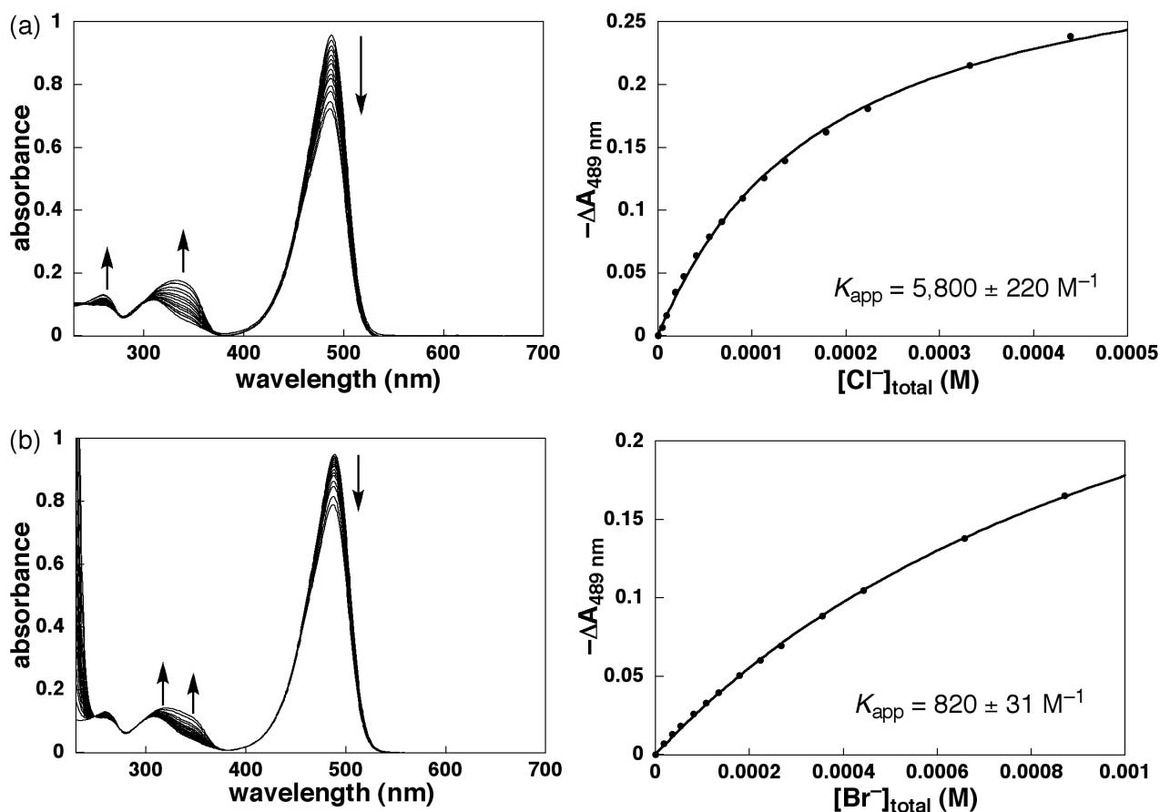
**Supporting Figure 6** UV-vis absorption spectral changes (left) and corresponding titration plots and 1:1 binding fitting curves (right) of **3a** ( $3.0 \times 10^{-6} \text{ M}$ ) upon the addition of (a) Cl<sup>-</sup> and (b) Br<sup>-</sup> as TBA salts in CH<sub>2</sub>Cl<sub>2</sub>.
