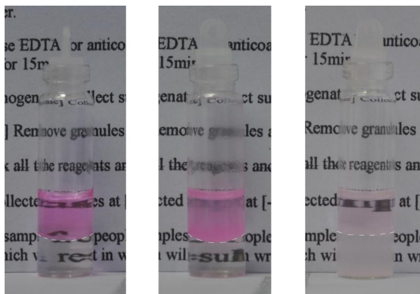
Figure S4. Phase transportation of dil-C18 from cyclohexane to water by taking on the Janus micro-reactor. Left: Dil-C18 cyclohexane solution over water. Middle: Soon after the addition of Janus micro-reactor to the cyclohexane phase of dil-C18 solution, the transparent oil phase becomes turbid. However the microspheres only stay in the oil phase shortly, before they start to settle down to the bottom layer of the oil phase. Right: The microspheres transfer into the water phase within 30 min. At this time point, it is noted that the bottom water phase become colourful turbid but homogeneous, whereas the top oil phase appears transparent again. Dash lines indicate the oil/water interface.
