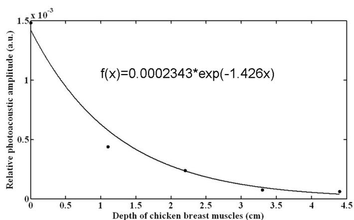
**Fig. S4** Experimental photoacoustic signal intensity of  $100 \mu\text{g mL}^{-1}$  PB NPs contained in agar gel embedded in chicken breast muscle measured at a wavelength of 765 nm as a function of depth from the laser-illuminated surface.
