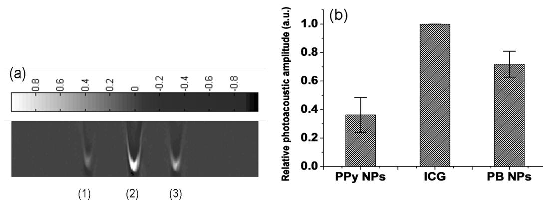
**Fig. S1** (a) Photoacoustic images of the aqueous (1) PPy NPs, (2) ICG and (3) PB NPs with the same concentration of 0.2 mg/mL. (b) Quantitative analysis of the photoacoustic amplitude which were corresponding to (a) (Note that the data were normalized to ICG).
