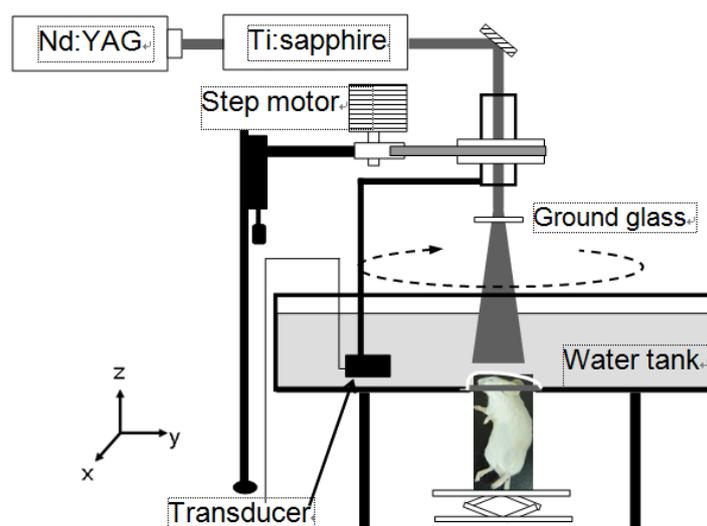
**Fig. S5** Schematic illustration of the PAT system for the in vivo imaging. Laser beamform: Orthogonal PAT design, which means the laser illumination passing through a ground glass, was orthogonal to ultrasound detection plane. Scanning step: the transducer scanned the object evenly along a horizontal circle trajectory, and signals were obtained every  $2.7^\circ$  with averaging 16 times.
