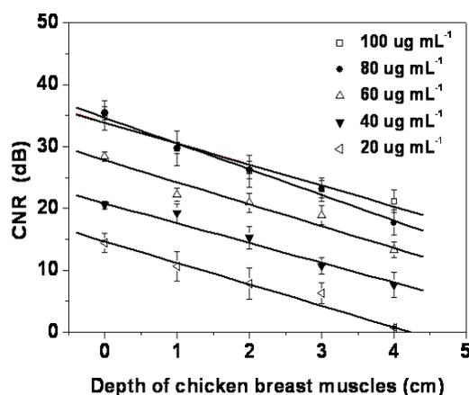
**Fig. S3** Plot of CNR in decibels as a function of depth of chicken breast muscles.
