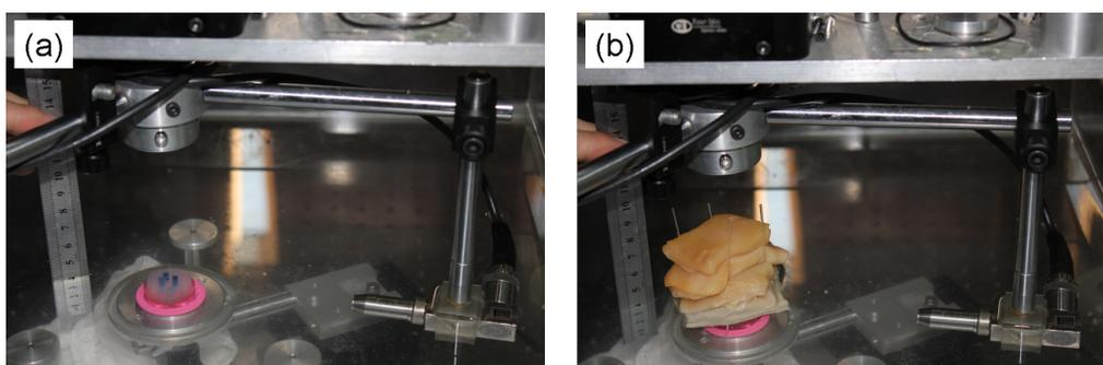
**Fig. S2** Experiment setup (a) The cross section of agar gels containing PB NPs with different concentration. (b) Stacked chicken breast muscle blocks on the PB NPs contained agar gels.
