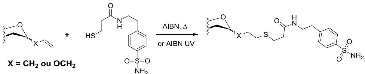
To a solution of 0.1 mmol of 1-O-allyl or 1-C-allyl sugar (1 equiv.) and 288mg of compound 7 (1mmol, 10 equiv.) in 10ml of 1,4-dioxane were added under argon atmosphere 33mg of AIBN. The mixture was then or refluxed for 20 hours, or irradiated under UV at 254nm for 7 hours. The mixture was then concentrated under vacuum and the residue purified on silica gel (methylene chloride – methanol 9.5 – 0.5, v-v).
