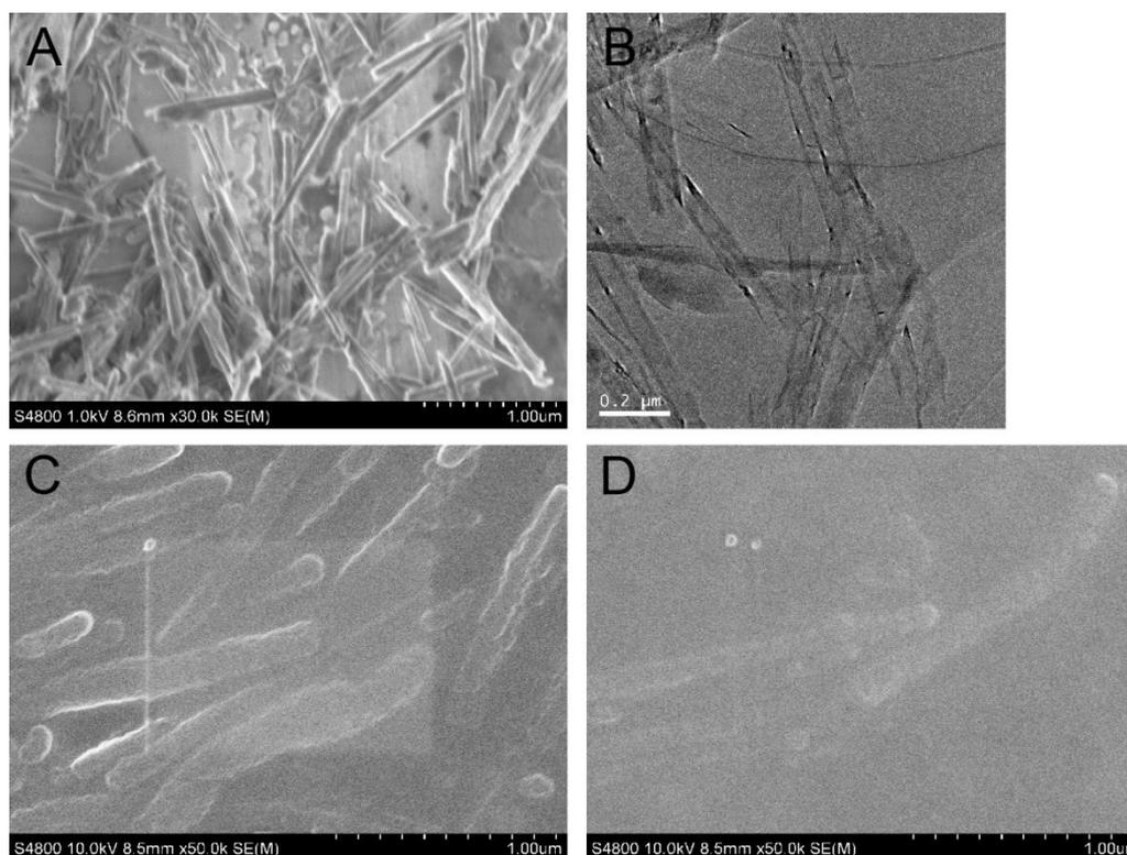
Fig S1. SEM (A) and TEM (B) images of BNNT; SEM images of BNNT@ MS (C) and BNNT-MS-NH<sub>2</sub> (D).
