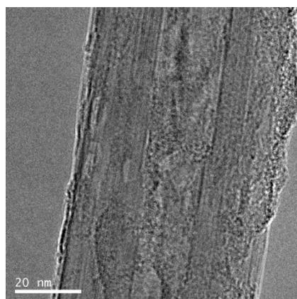
Fig S2. TEM image of a hydrogen peroxide BNNT @ MS hybrid.
