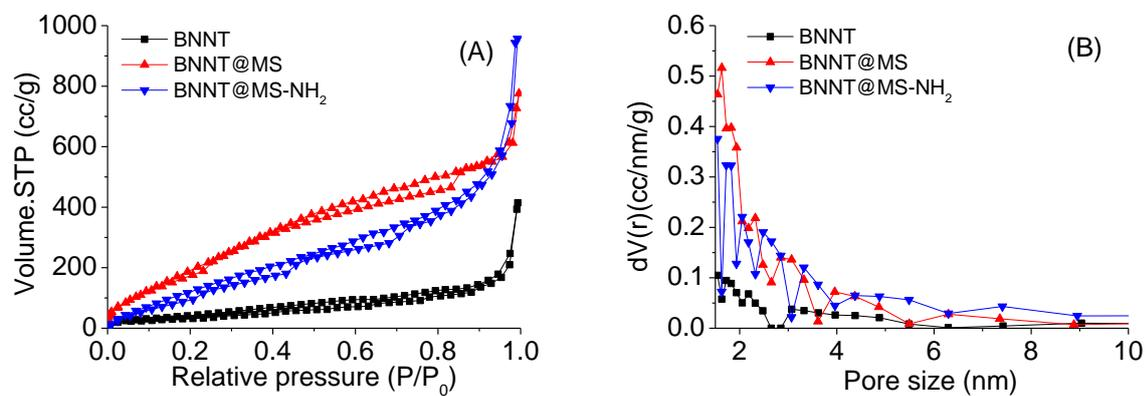
Fig S3. N<sub>2</sub> adsorption-desorption isotherms (A) and pore size distribution (B) of various samples.
