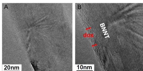
**Fig S5.** Low- (A) and high- (B) magnification TEM images of BNNTs loaded with dox.
