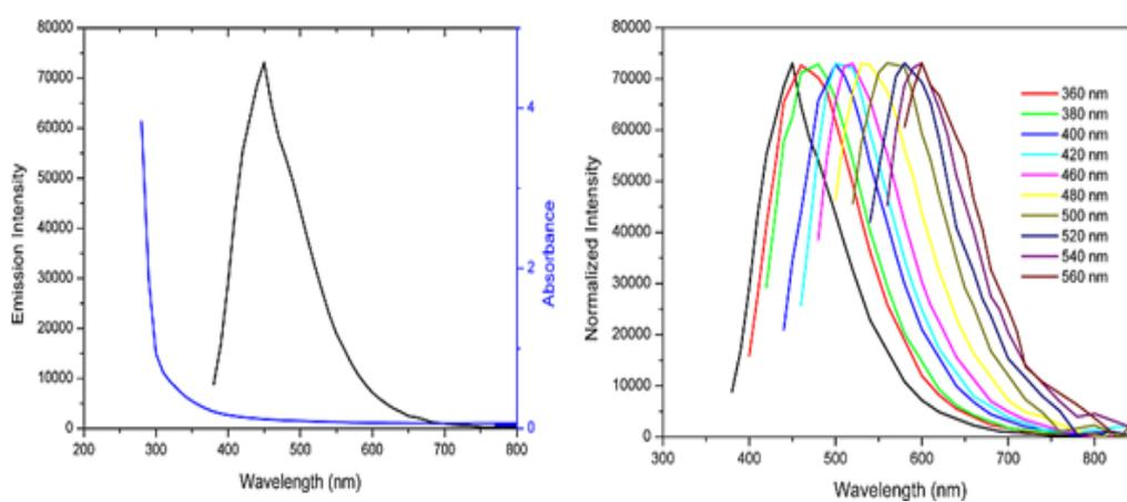
**Figure. S3.** (a) UV/Vis absorption, emission spectra (excitation at 360 nm) and normalized emission spectra of the gC-Dots (b) UV/Vis absorption, emission spectra (excitation at 360 nm) and normalized emission spectra of the SH-gC-Dots.
