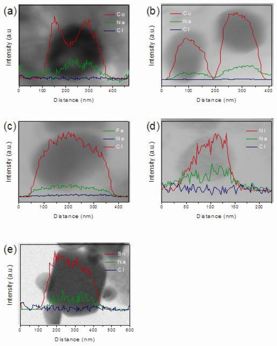
**Fig. S1** Typical linescan analyses of (a) NaBH<sub>4</sub>@Co, (b) NaBH<sub>4</sub>@Cu, (c) NaBH<sub>4</sub>@Fe, (d) NaBH<sub>4</sub>@Ni, and (e) NaBH<sub>4</sub>@Sn. No Cl was detected over any of the individual core-shell nanoparticles.
