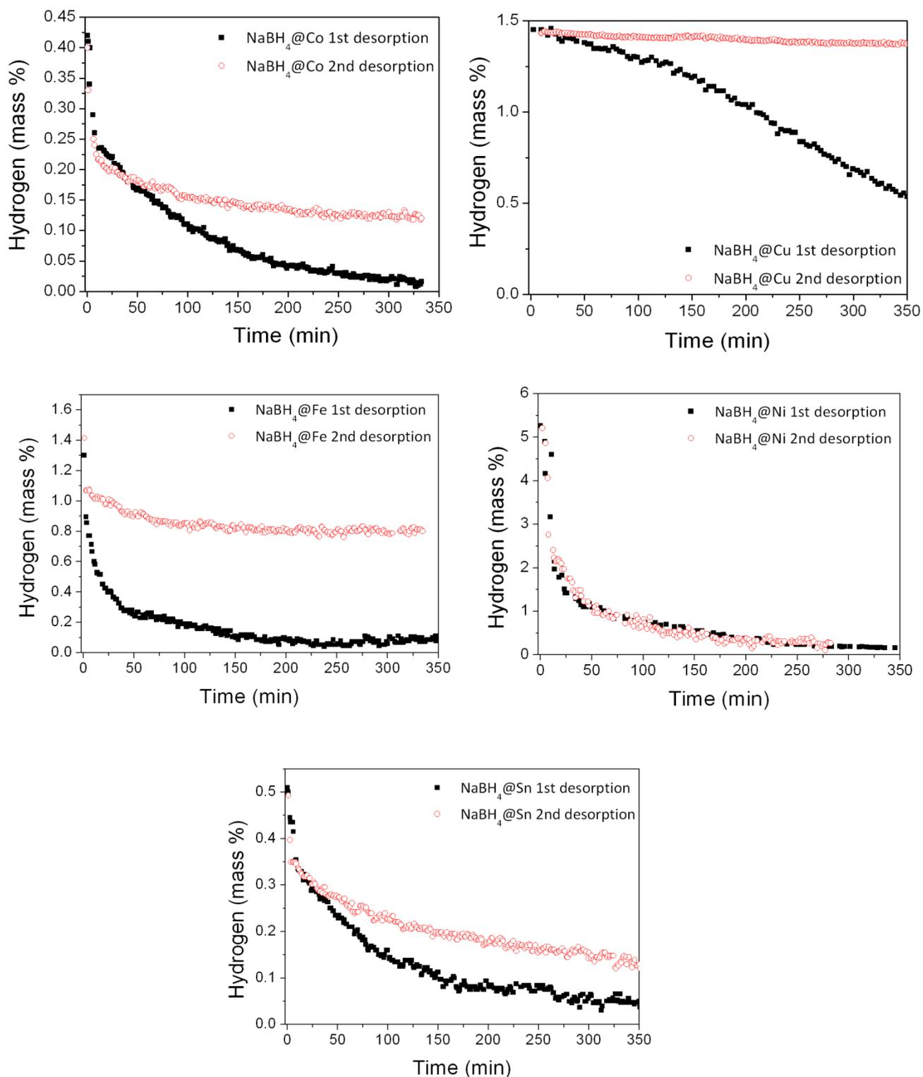
**Fig. S7** Kinetics of successive hydrogen desorption at 0.01 MPa and 350 °C from (a) NaBH<sub>4</sub>@Co, (b) NaBH<sub>4</sub>@Cu, (c) NaBH<sub>4</sub>@Fe, (d) NaBH<sub>4</sub>@Ni, and (e) NaBH<sub>4</sub>@Sn. Hydrogen absorption was performed under 40 MPa hydrogen pressure (not shown).
