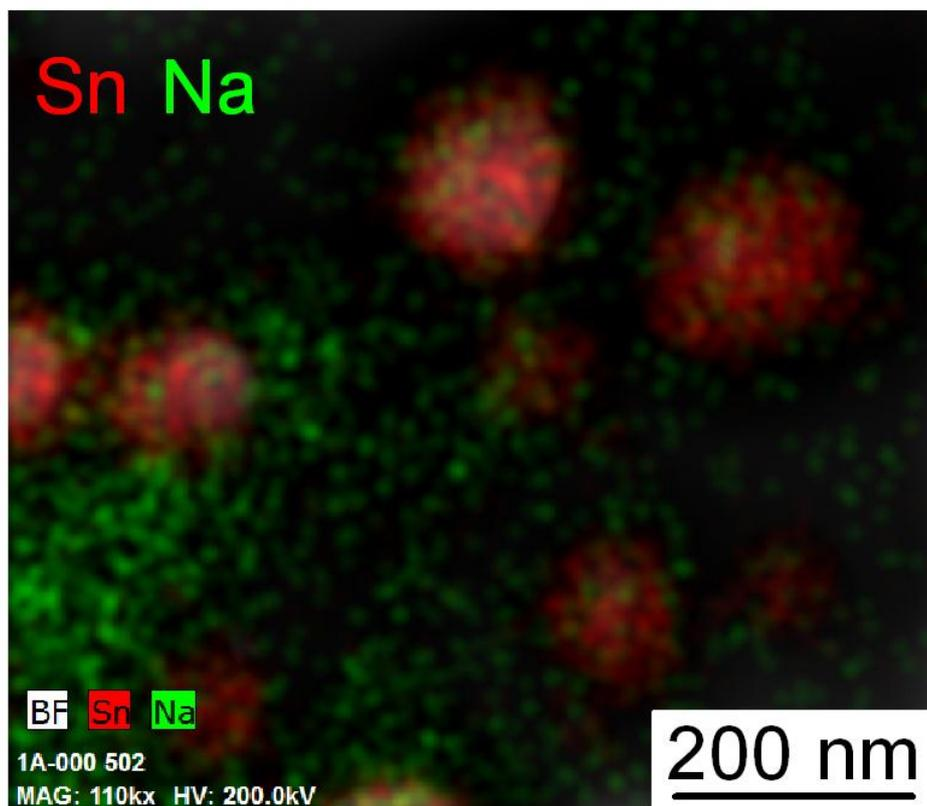
**Fig. S6** Typical EDS mapping of NaBH<sub>4</sub>@Sn heated to 300 °C showing the degradation of the original cubic-like structure to form a combination of spherical Sn nanoparticles and NaBH<sub>4</sub>.
