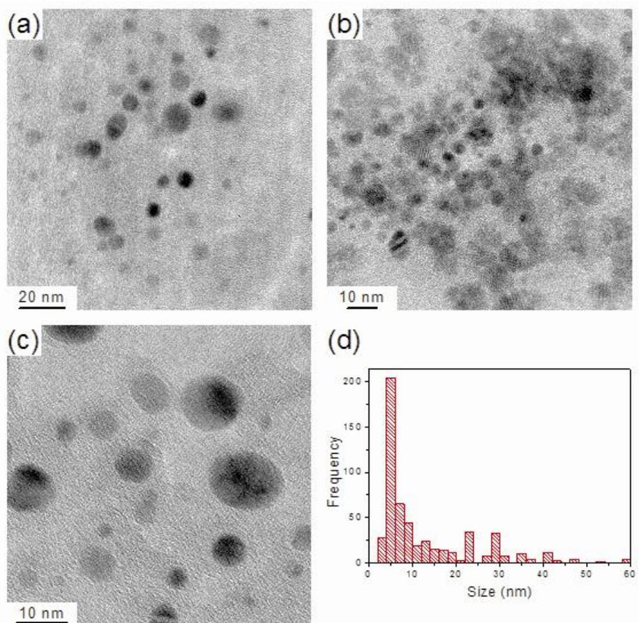
**Fig. S2** (a)-(c) Typical TEM images of NaBH<sub>4</sub> nanoparticles before metal coating, and (d) typical size distribution as observed across the range of samples analysed by TEM.
