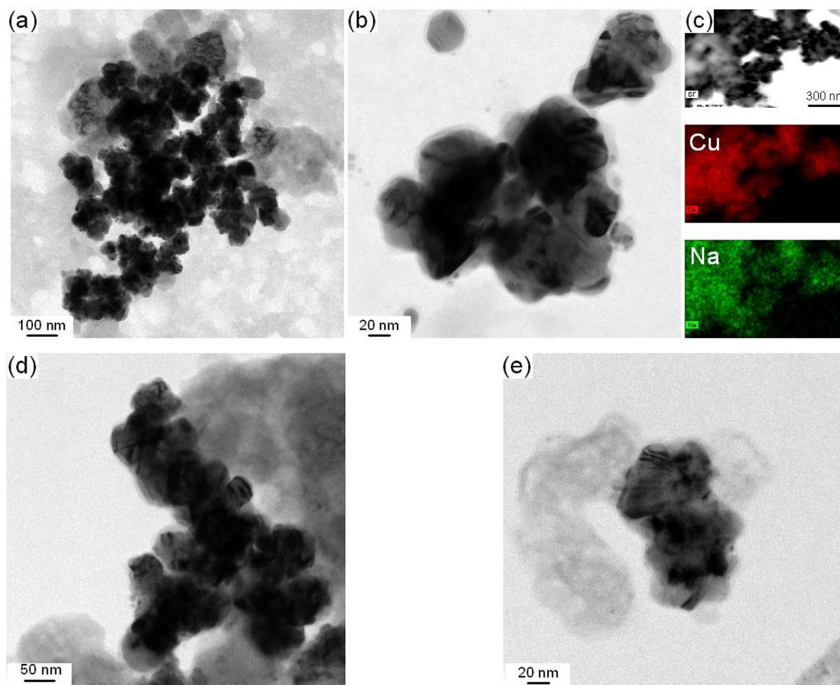
**Fig. S4** (a)-(e) Typical TEM images of  $\text{NaBH}_4@\text{Cu}$  produced from  $0.06 \text{ mol.L}^{-1} \text{ CuCl}_2$  and (c) associated EDS mapping showing the formation of an irregular Cu surface at high  $\text{CuCl}_2$  concentrations.
