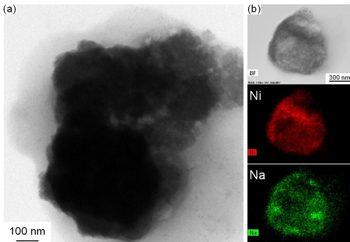
**Fig. S3** (a) Typical TEM image of NaBH<sub>4</sub>@Ni produced from 0.02 mol.L<sup>-1</sup> NiCl<sub>2</sub> and (b) associated EDS mapping of the large particle/agglomerate (a), showing a combination of agglomerated Ni and NaBH<sub>4</sub>.
