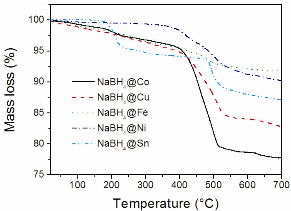
**Fig. S5** TGA curves for the core-shell nanoparticles under a heating ramp of 10 °C.min<sup>-1</sup>.
