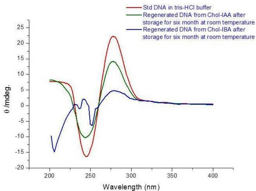
*Fig. S6.* CD spectra of regenerated DNA in chol-IAA and chol-IBA stored for six months along with standard DNA in Tris-HCl buffer.
