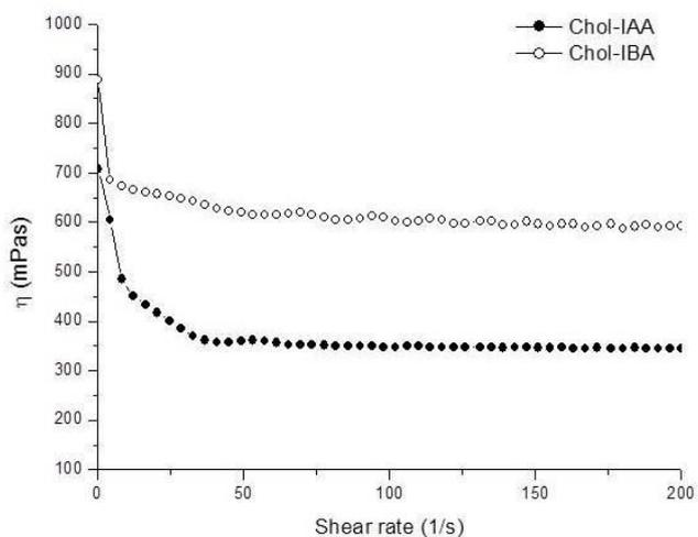
**Figure S2** : Steady shear viscosity of chol-IAA and chol-IBA ionic liquids.
