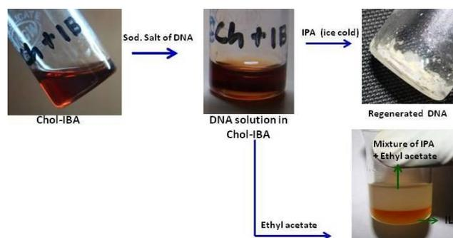
**Fig. S3:** Dissolution of sodium salt of DNA in chol-IBA. Pictorial demonstration of the recycling of the IL
