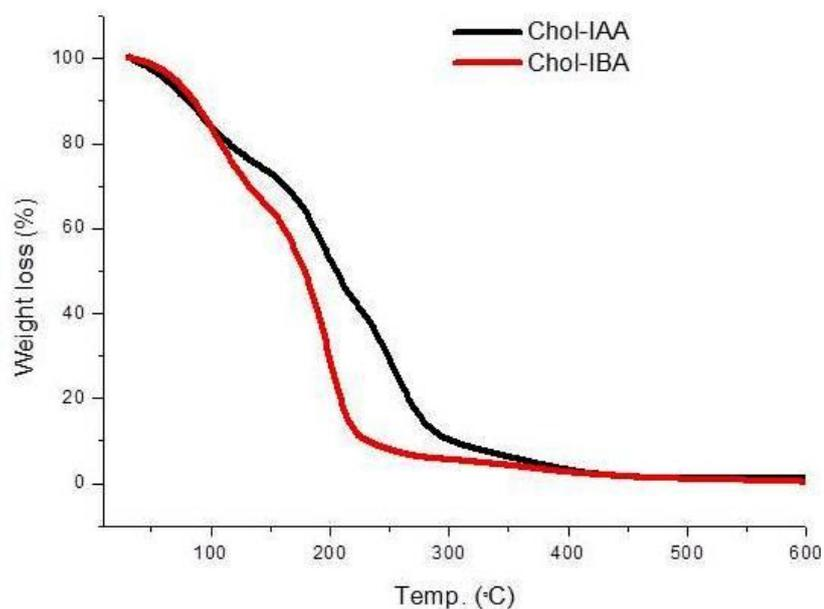
**Fig. S1**: TGA thermogram of chol-IAA and chol-IBA ionic liquids.
