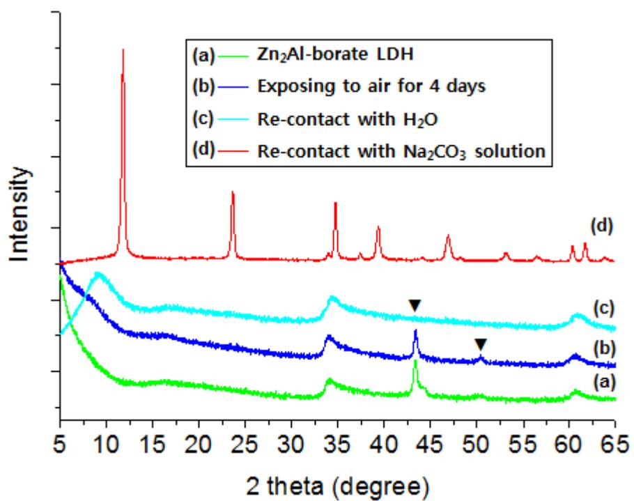
**Figure S1.** XRD patterns of acetone washed  $Zn_2Al$ -borate LDH (a) dried powder, (b) exposed to air for 4 days, (c) re-contacted with  $H_2O$ , and (d) re-contact with  $Na_2CO_3$  solution. (▼) reflections from the sample holder.
