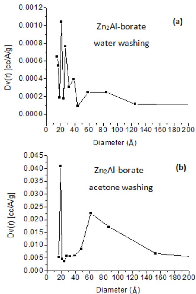
**Figure S9.** Pore size distribution of Zn<sub>2</sub>Al-borate washed with (a) water and (b) acetone.
