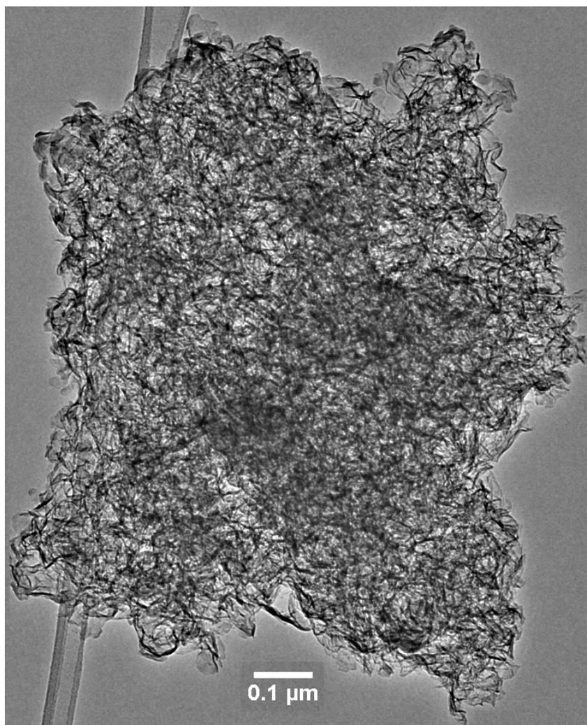
**Figure S5.** TEM image of Zn<sub>2</sub>Al-borate LDH prepared by AMOST method.
