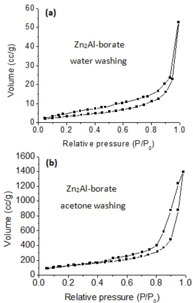
**Figure S8.** BET N<sub>2</sub> isotherms for Zn<sub>2</sub>Al-borate LDHs washed with (a) water, and (b) acetone.
