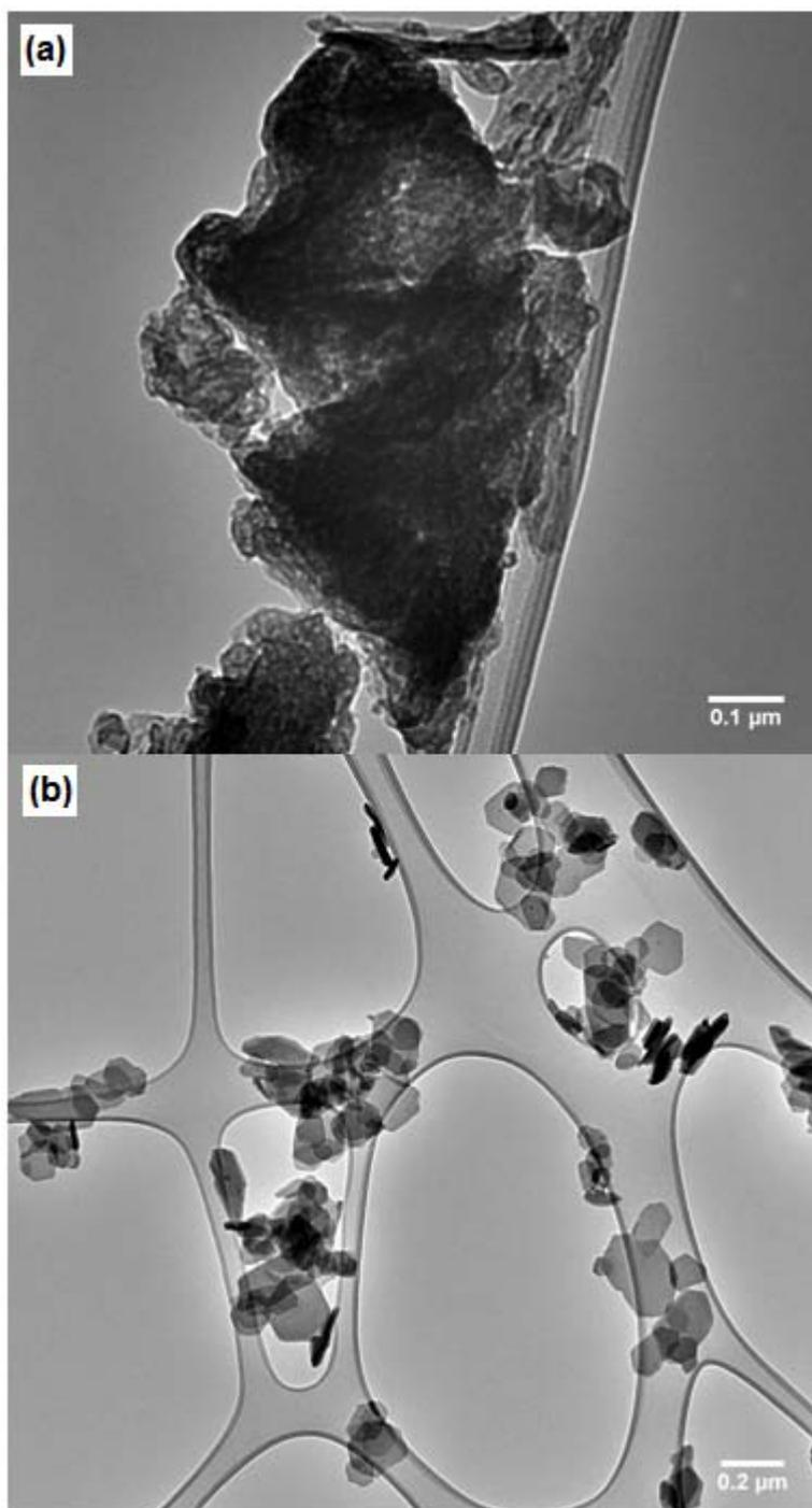
**Figure S2.** TEM image of acetone washed Zn<sub>2</sub>Al-borate LDH after re-contacting with (a) H<sub>2</sub>O and (b) Na<sub>2</sub>CO<sub>3</sub> aqueous solution.
