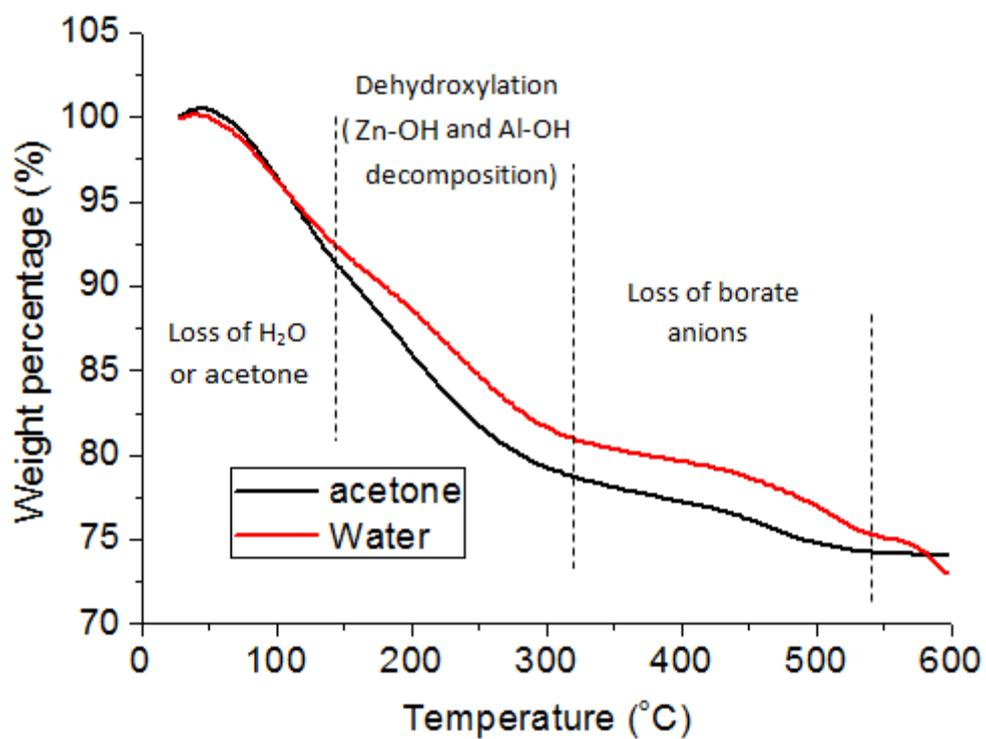
**Figure S10.** TGA analysis of Zn<sub>2</sub>Al-borate washed with (a) acetone or (b) water.
