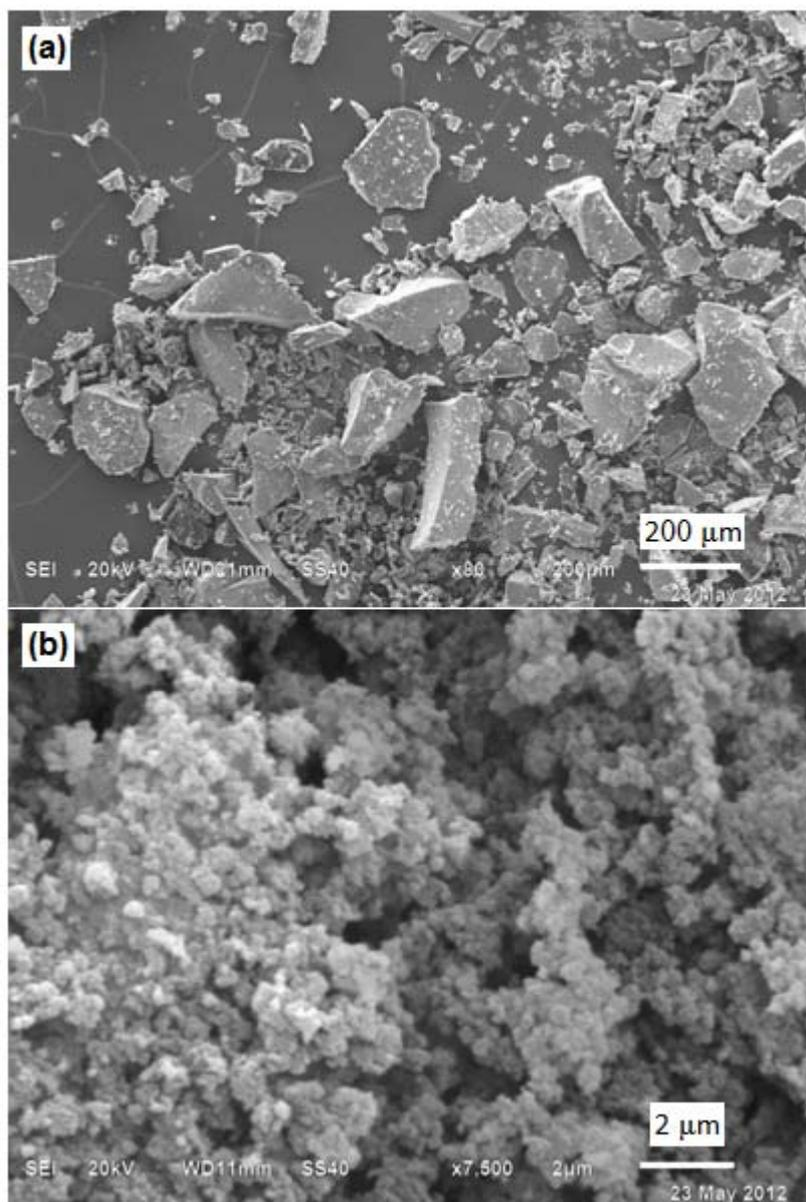
**Figure S7.** SEM images of Mg<sub>3</sub>Al-borate LDH washed with (a) water and (b) acetone.
