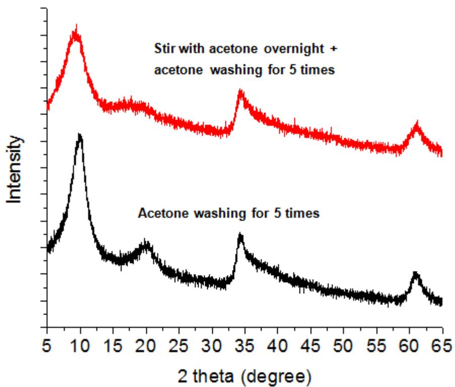
**Figure S11.** XRD patterns of water washed  $Zn_2Al$ -borate LDH dry powder that (a) stirred with acetone overnight + acetone washing for 5 times, and (b) acetone washing for 5 times.
