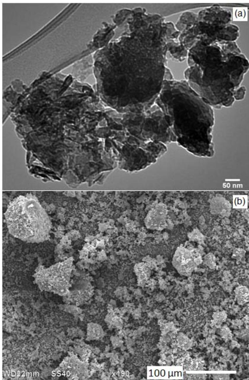
**Figure S4.** (a) TEM and (b) SEM images of Zn<sub>2</sub>Al-borate LDH synthesized by conventional co-precipitation.
