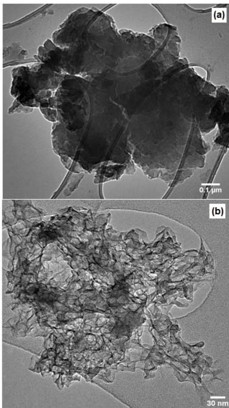
**Figure S6.** TEM images of Mg<sub>3</sub>Al-borate LDHs washed with (a) water and (b) acetone.
