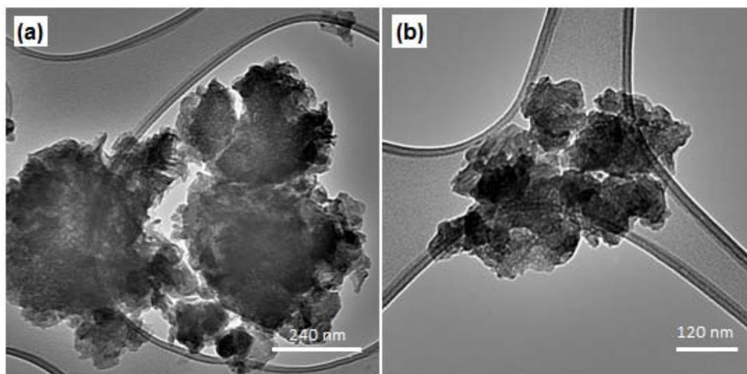
**Figure S12.** TEM images of water washed  $\text{Zn}_2\text{Al}$ -borate LDH dry powder that (a) stirred with acetone overnight + acetone washing for 5 times, and (b) acetone washing for 5 times.
