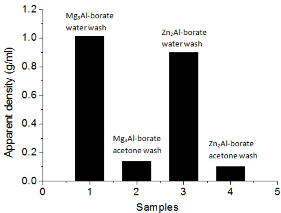
**Figure S3.** Apparent density of Mg<sub>3</sub>Al-borate and Zn<sub>2</sub>Al-borate washed with water or acetone.
