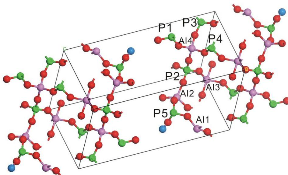
Fig.S3. the crystal structure of Mu-4. Green: P, Purple: Al, Red: O, Blue: H.
