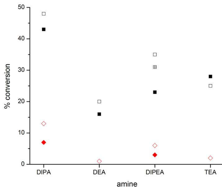
**Fig. S-3** Effects of changing amine on the conversion of fcI<sub>2</sub> to fcI(C≡CPh) (black squares) and fc(C≡CPh)<sub>2</sub> (red diamonds), entries 6-9, Table S-3. Solid symbols = run 1, open symbols = run 2, crossed symbols = run 3 (DIPEA only).
