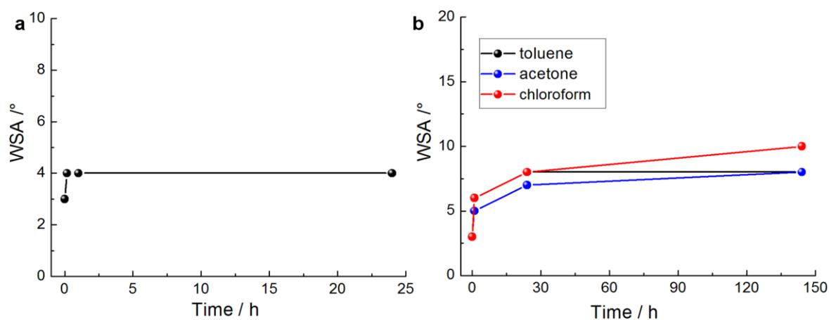
**Fig. S13.** Variation of WSA of water drops (10µL) on the superhydrophobic textile with (a) UV irradiation time and (b) immersion time in organic solvents.
