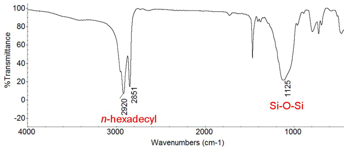
**Fig. S7.** IR spectrum of the residue after dip coating of a fabric in the HD-oligomer/HD-silica nanocomposite dispersion.
