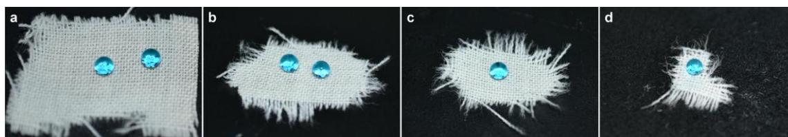
**Fig. S10.** Images of the coated wool fabrics after (a) 10, (b) 30, (c) 50 and (d) 100 cycles of abrasion at 5.0 kPa using sandpaper as the abrasion partner.
