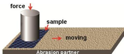
**Fig. S3.** Schematic illustration of the abrasion test employed to evaluate the mechanical durability of the samples.
