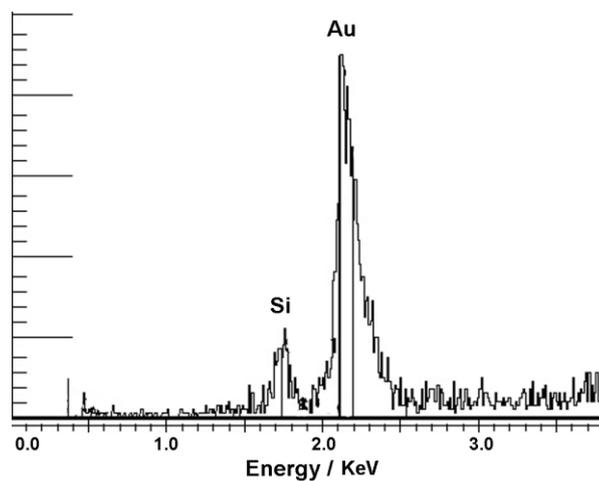
**Fig. S12.** EDX spectrum of the coated wool fabric after 200 cycles of abrasion at 5 kPa.
