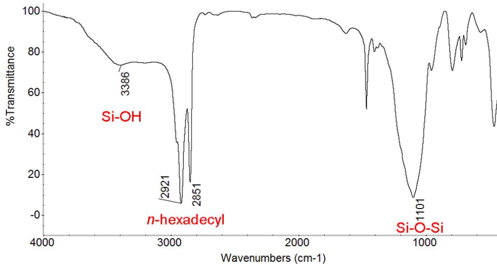
**Fig. S5.** IR spectrum of the HD-oligomer/HD-silica nanocomposite.
