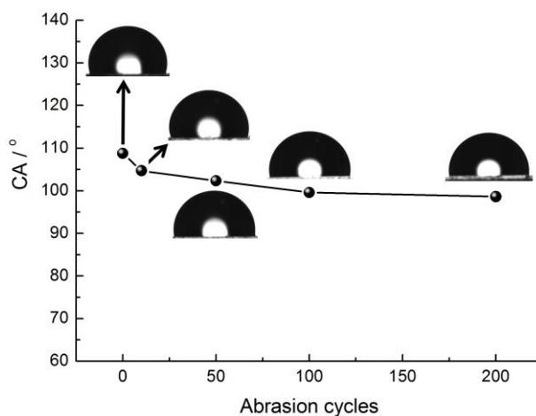
**Fig. S11.** CA changes depending on abrasion cycles (40cm each) at 5.0 kPa by using the glass slide as the substrate.
