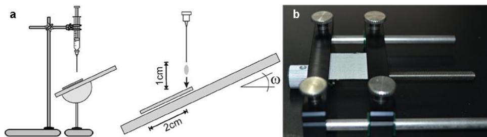
**Fig. S2.** (a) Principle setup employed for measuring SHA ( $\omega$ ) (3) and (b) the sample holder.
