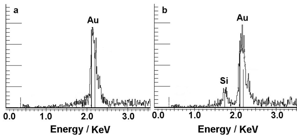
**Fig. S8.** EDX spectra of the (a) pristine and (b) coated wool fabrics.
