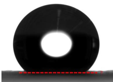
**Fig. S1.** Typical image of a water droplet on the superhydrophobic textile.
