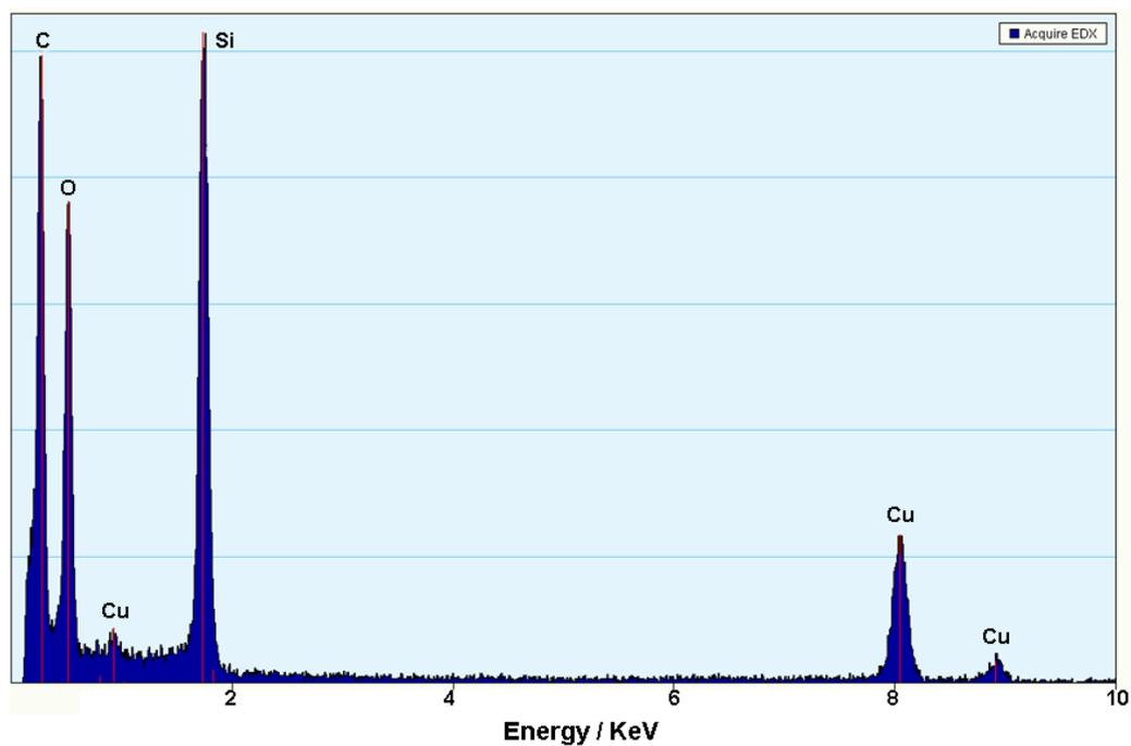
**Fig. S6.** EDX spectrum of the HD-oligomer/HD-silica nanocomposite.
