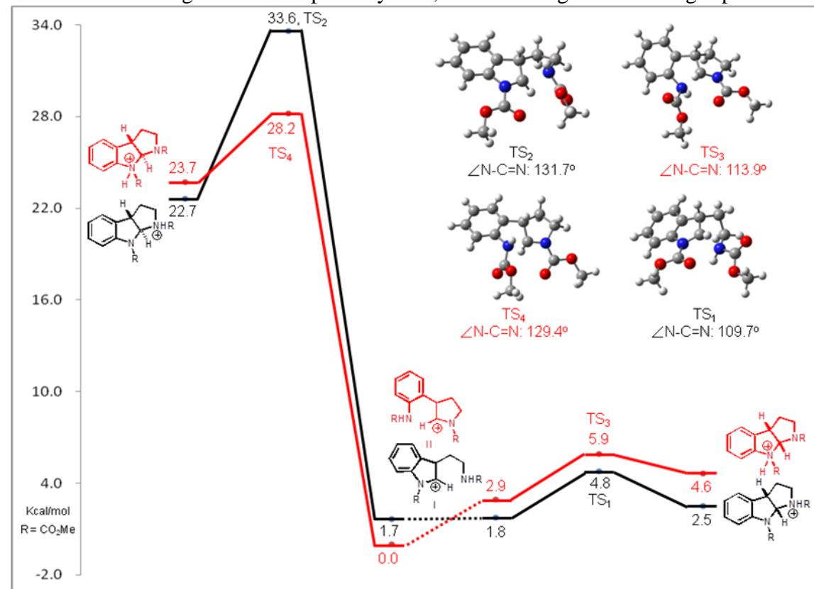
Scheme 2: PES diagrams of four pathways 1-4, and the TSs geometries in acetonitrile:
