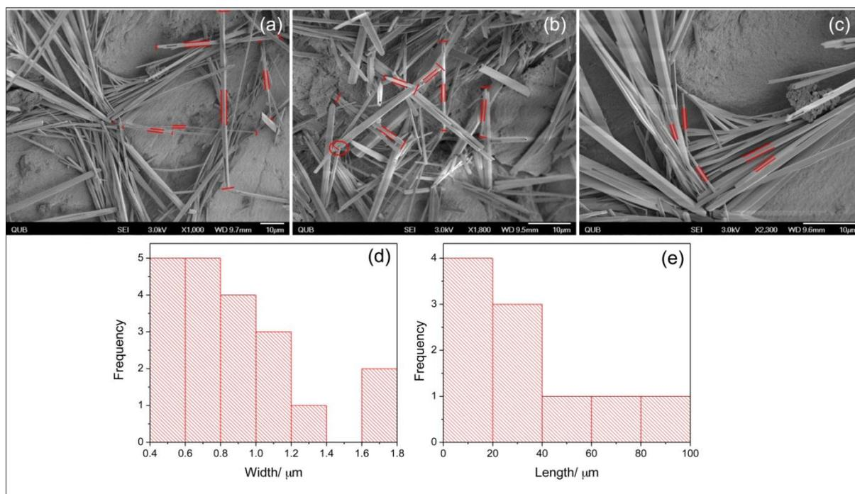
**Figure S4.** (a-c) Representative SEM images of PFO-OG-Si microtubes (PFO/sorbitol gelator transcribed with silica) prepared from different synthesis batches. Samples aged for 14 weeks. (d) and (e) show the corresponding width and length distributions of PFO-OG-Si microtubes across all batches.
