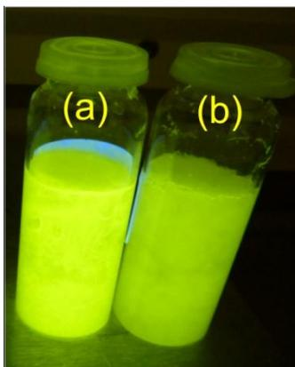
**Figure S1.** Observed photoluminescence from (a) PFO-OG and (b) PFO-OG-Si under UV excitation (366 nm).
