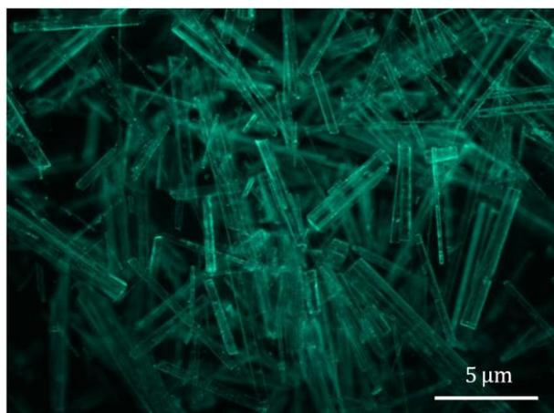
**Figure S8.** Fluorescence microscopy image of PFO-OG ( $\lambda_{\text{ex}} = 360\text{-}370\text{ nm}$ , 10x magnification)
