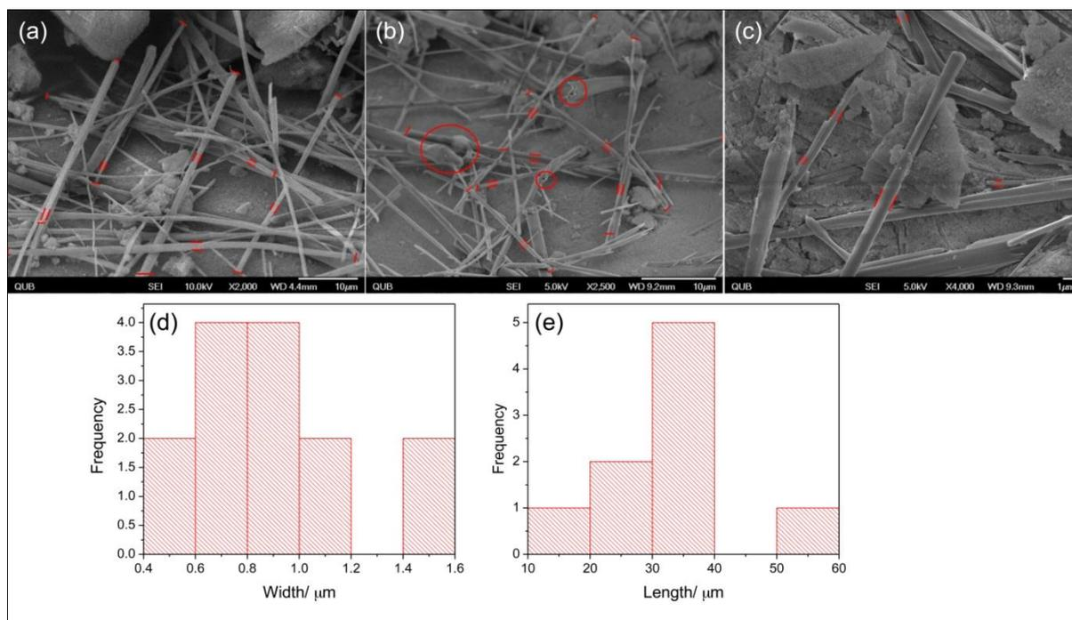
**Figure S3.** (a-c) Representative SEM images of OG-Si microtubes (sorbitol gelator transcribed with silica) prepared from different synthesis batches. Samples aged for 14 weeks. (d) and (e) show the corresponding width and length distributions of OG-Si microtubes across all batches.
