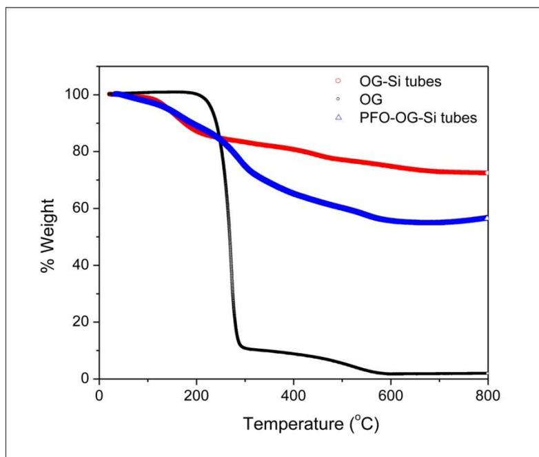
**Figure S6.** Thermogravimetric analysis (TGA) of (a) OG-Si, (b) OG and (c) PFO-OG-Si.
