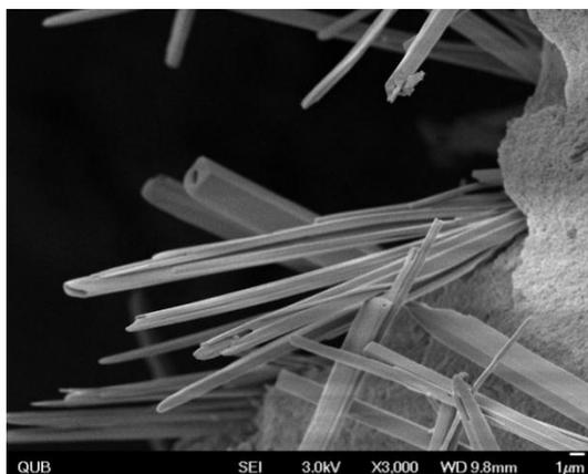
**Figure S2.** Representative SEM image of PF-OG-Si microtubes.
