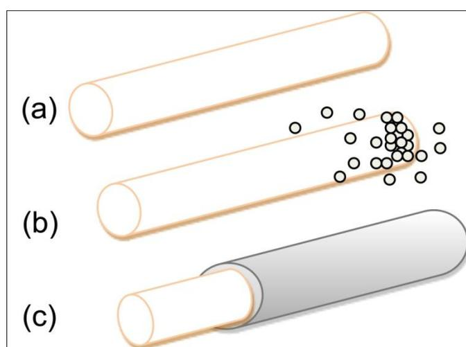
**Figure S9.** Schematic representation of transcription of an organogel with silica: (a) self-assembled organic fibre; (b) deposition of silica sol from suspension and (c) condensation and structural consolidation of silica around the organic template.
