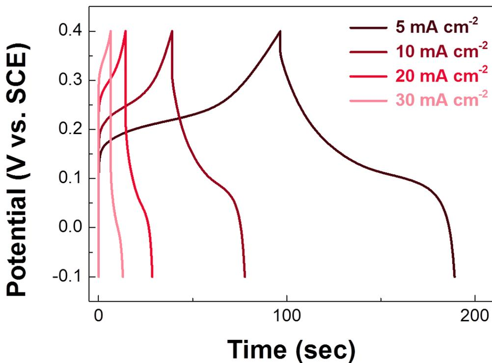
**Fig. S4.** The galvanostatic charge-discharge curves of the Co-Ni multiphase composite film at various current densities.
