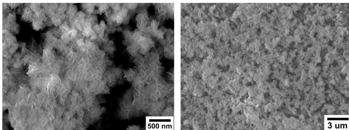
**Fig S2.** SEM images of the Co-Ni multiphase composite film showing its a corrugated morphology.
