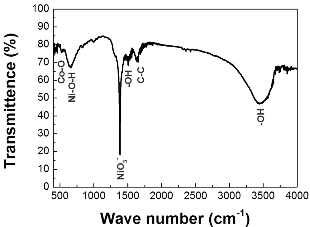
**Fig S3.** FTIR spectra of the Co-Ni multiphase composite film. Co-O, Ni-O-H, NiO<sub>3</sub><sup>-</sup> and -OH groups appear around at 520 cm<sup>-1</sup>, 660 cm<sup>-1</sup>, 1380 cm<sup>-1</sup>, 3400 cm<sup>-1</sup> and 1500 cm<sup>-1</sup>, respectively.
