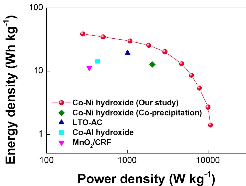
**Fig. S5.** Ragone plot representing the energy and power density in a supercapacitor of the Co-Ni multiphase composite film compared with those of other composite materials fabricated by various methods for supercapacitor
