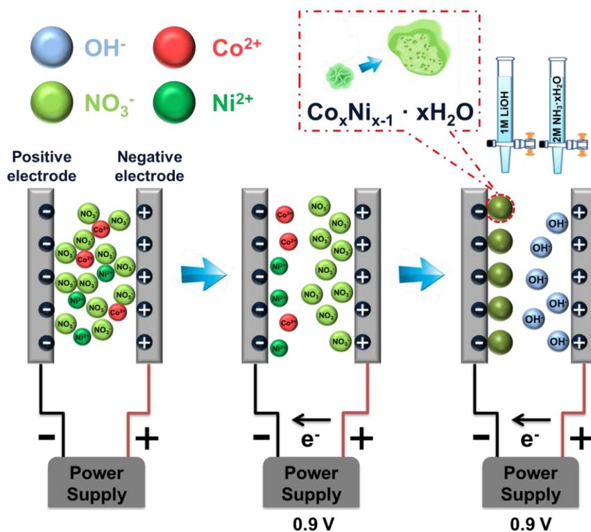
**Fig. S1.** Schematic drawing of the Co-Ni multiphase composite film and its synthetic process based on the novel co-precipitation method.
