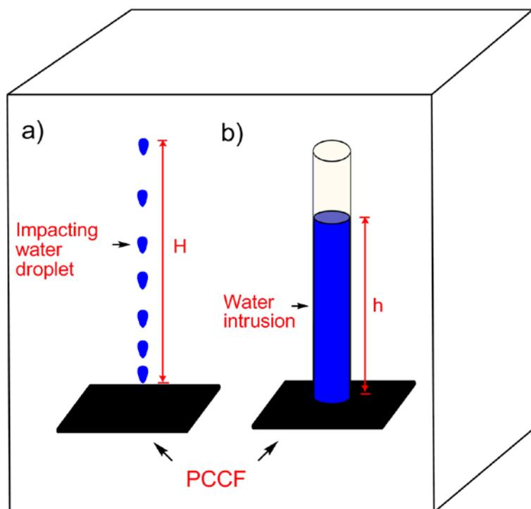
Fig. S5 Schematic illustration of the critical water impact dynamic pressure (a) and water intrusion pressure (b) on PCCF.
