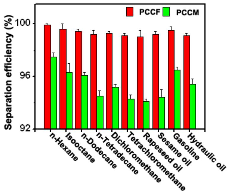
Fig. S4 The separation efficiency of PCCF and PCCM for a selection of oils.
