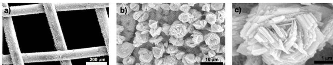
**Fig. S1** SEM images of the CuO-grown copper mesh at low resolution (a), at higher resolution (b), and close-up image of an individual flower-like spherical structure (c).
