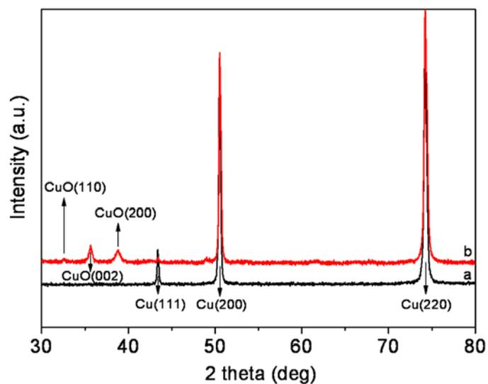
**Fig. S2** XRD patterns of Cu (a) and CuO-grown Cu (b).
