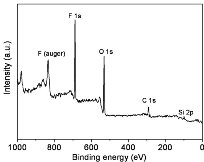
**Fig. S3** XPS survey spectra for the surface of the PFTS-modified CuO-grown copper sample.
