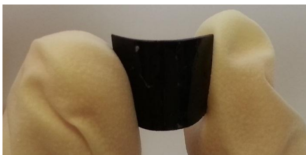
Figure S10. Photo showing the flexibility of one of the films used for electrical conductivity test.
