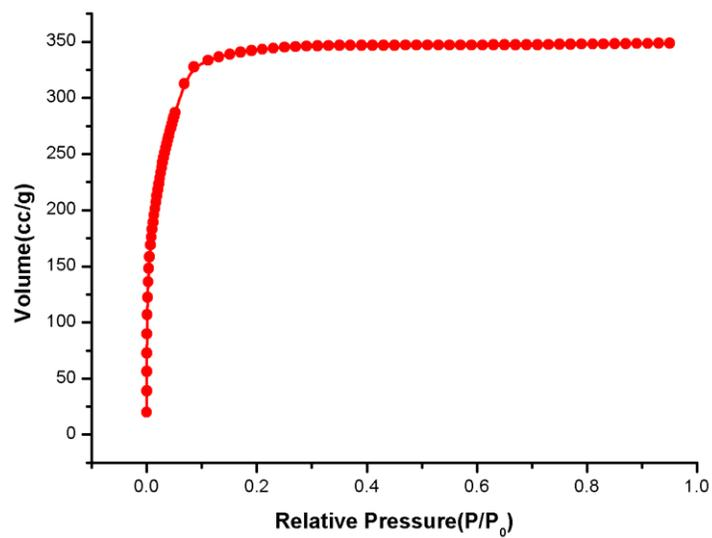
Figure 12 . N<sub>2</sub> adsorption isotherm of ocMOM-1 at 77K;
