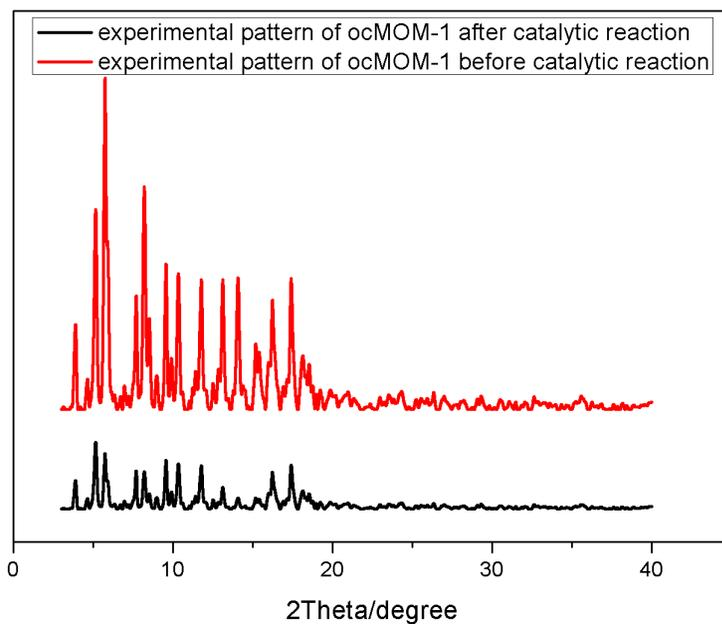
Figure S10. Comparison of experimental XPRD pattern of ocMOM-1 before and after catalytic reaction.
