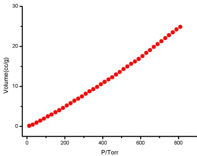
Figure 13. CO<sub>2</sub> adsorption at 273K.
