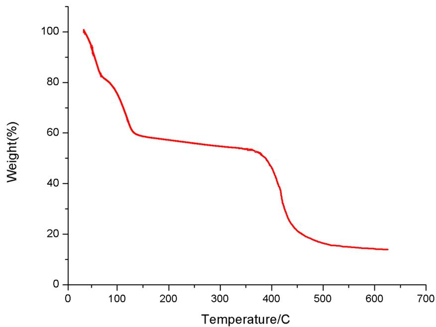
Figure S6. Thermogravimetric analysis of ocMOM-2
