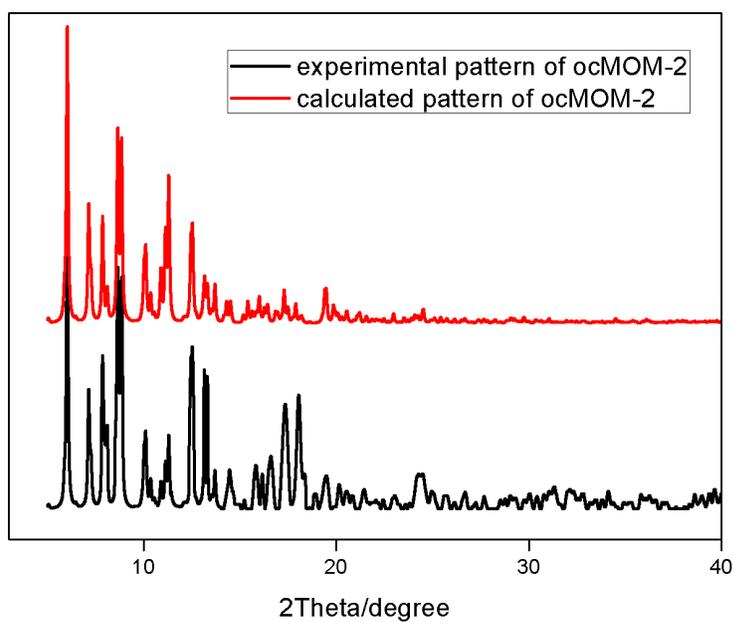
Figure S4. Comparison of experimental and calculated powder x-ray diffraction patterns of ocMOM-2
