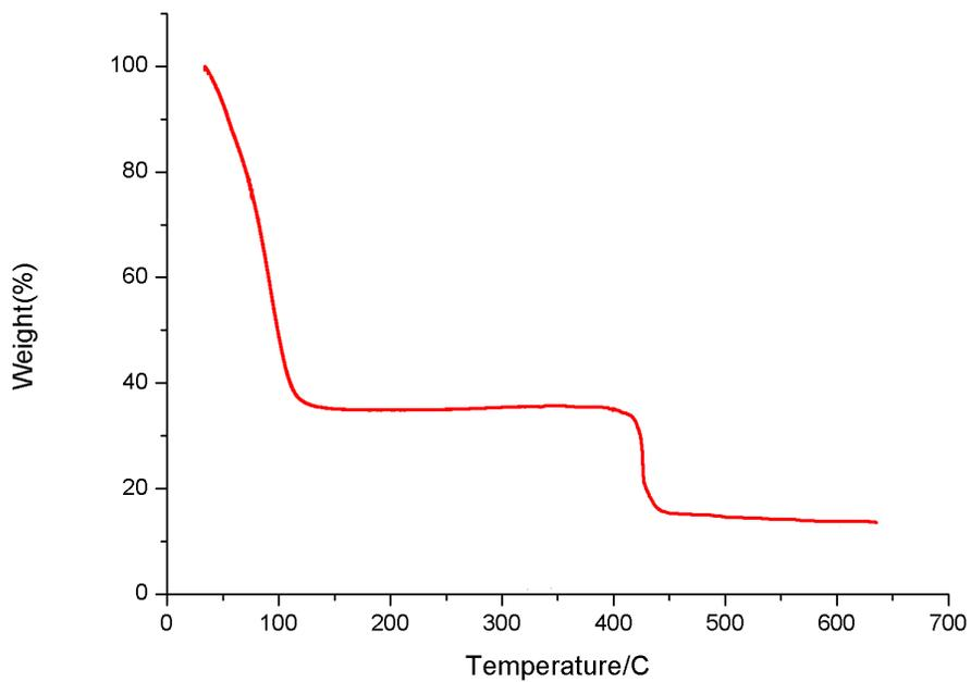
Figure S3. Thermogravimetric analysis of ocMOM-1
