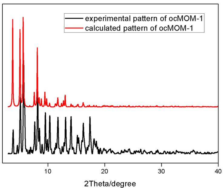
Figure S1. Comparison of experimental and calculated powder x-ray diffraction patterns of ocMOM-1
