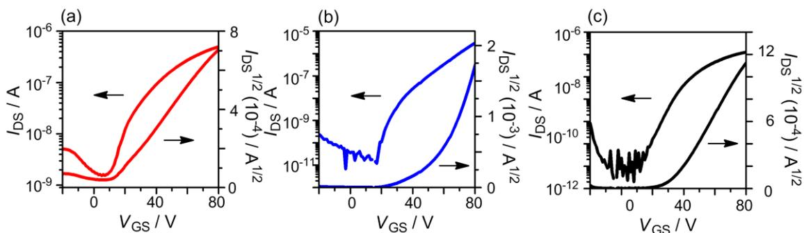
**Fig. S5** Transfer characteristics of OFETs based on (a) **Tetra-PDI**, (b) **Hexa-PDI**, and (c) **6** at a drain voltage of 80 V.
