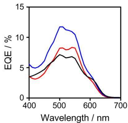
**Fig. S3** EQE spectra of the OPV devices based on blend of P3HT:**Tetra-PDI** (red solid line), P3HT:**Hexa-PDI** (blue solid line), and P3HT:**6** (black solid line).
