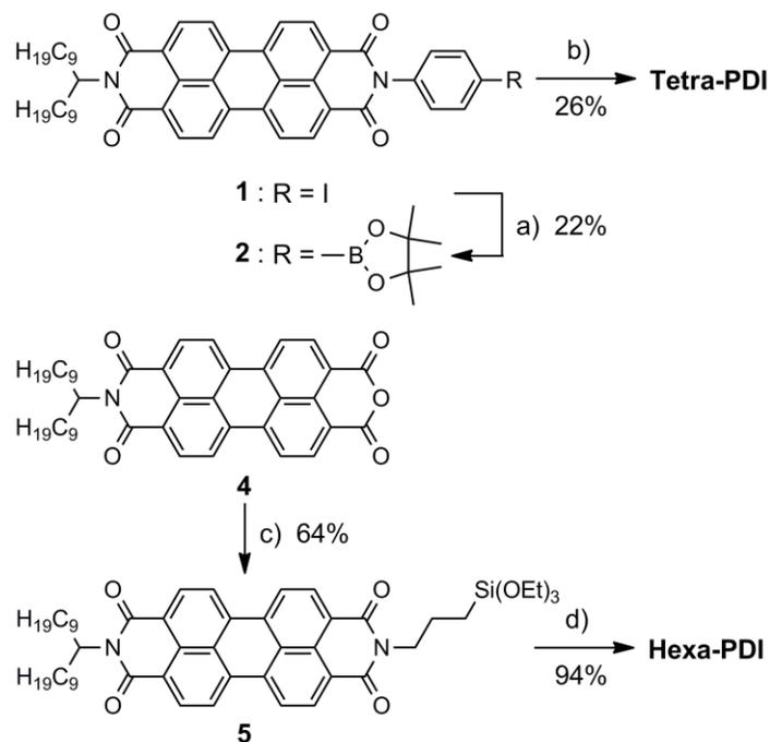
**Scheme S1.** Syntheses of **Tetra-PDI** and **Hexa-PDI**. Reagents and conditions: (a)  $\text{PdCl}_2(\text{dppf})$ , KOAc, bis(pinacolato)diboron, DMSO, 110 °C; (b)  $\text{Pd}(\text{PPh}_3)_4$ ,  $\text{K}_2\text{CO}_3$ ,  $\text{C}(\text{C}_6\text{H}_4\text{I})_4$  (**3**), THF/ $\text{H}_2\text{O}$ , 90 °C; (c)  $\text{H}_2\text{N}(\text{CH}_2)_3\text{Si}(\text{OEt})_3$ , 150 °C; (d) TBAF,  $\text{CHCl}_3$ , r.t..
