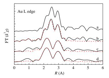
**Fig. S5.** Au  $L_3$  edge EXAFS of the Au foil (a),  $Au_{2.0}$ /Graphene (b), fresh  $Au_{2.0}$ -Pd<sub>1.0</sub>/Graphene (c) and spent  $Au_{2.0}$ -Pd<sub>1.0</sub>/Graphene (d) catalysts. Red dashed lines are those fitted for the first-shell.
