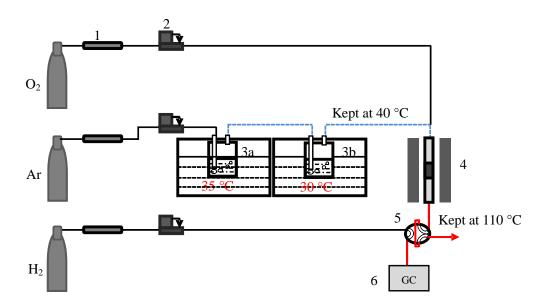
**Fig. S1.** Schematic setup of the apparatus for the catalytic tests of methanol selective oxidation: (1) Purification tube, (2) Mass flow controller, (3) Methanol saturator, (4) Fixed-bed reactor, (5) Six-way wave, and (6) Gas chromatograph.
