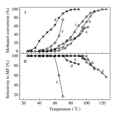
**Fig. S7.** Methanol conversion (I) and selectivity to MF (II) for methanol oxidation over the Au<sub>m</sub>-Pd<sub>n</sub>/Graphene catalysts with different Au/Pd loadings. (a) Au<sub>1.0</sub>-Pd<sub>0.5</sub>/Graphene, (b) Au<sub>1.0</sub>-Pd<sub>1.0</sub>/Graphene, (c) Au<sub>1.0</sub>-Pd<sub>2.0</sub>/Graphene, (d) Au<sub>2.0</sub>-Pd<sub>1.0</sub>/Graphene; and (e) Au<sub>4.0</sub>-Pd<sub>2.0</sub>/Graphene. Reaction conditions are the same as those listed in Fig. S4.
