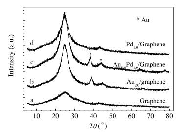
**Fig. S3.** XRD patterns of Graphene (a),  $Au_{2.0}$ /Graphene (b),  $Au_{2.0}$ -Pd<sub>1.0</sub>/Graphene (c), and Pd<sub>1.0</sub>/Graphene (d).
