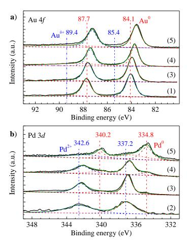
**Fig. S4.** Au 4f (a) and Pd 3d (b) XPS spectra of the Au<sub>2.0</sub>/Graphene (1), Pd<sub>1.0</sub>/Graphene (2), Pd<sub>1.0</sub>/Graphite (3), Au<sub>2.0</sub>-Pd<sub>1.0</sub>/CNTs (4), and Au<sub>2.0</sub>-Pd<sub>1.0</sub>/Graphene (5) catalysts. This Fig. is identical to Fig. 2 in the main manuscript.
