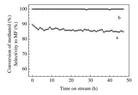
**Fig. S8.** Long-term test of the selective oxidation of methanol over  $Au_{2.0}$ - $Pd_{1.0}$ /Graphene at 70 °C: (a) methanol conversion; (b) selectivity to MF. Reaction conditions: 60 mg catalyst; feed of 6.4 vol.% CH<sub>3</sub>OH + 70.2 vol.% O<sub>2</sub> + balanced Ar with a flow rate of 42.5 ml/min.
