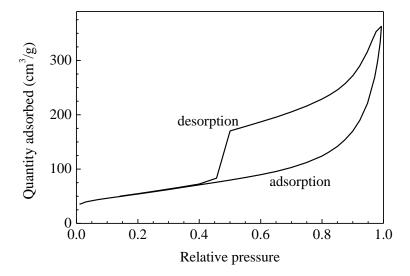
Fig. S2. Nitrogen adsorption and desorption isotherms of the  $Au_{2.0}$ -Pd<sub>1.0</sub>/Graphene catalyst.
