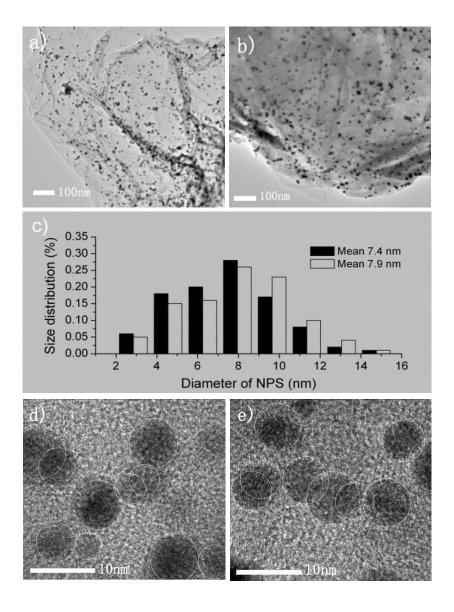
**Fig. S9.** Representative TEM images and size distribution of Au<sub>2.0</sub>-Pd<sub>1.0</sub>/Graphene. (a) Fresh catalyst; (b) Spent catalyst; (c) Size distribution of Au and Pd nanoparticles (the solid bars for the fresh catalyst, while the open bars for the spent catalyst after 48 h long-term test for methanol oxidation); d) HR-TEM of the fresh catalyst; e) HR-TEM of the spent catalyst.
