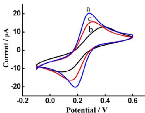
**Fig. S1** Cyclic voltammograms of 1 mM  $[\text{Fe}(\text{CN})_6]^{3-/4-}$  on a bare gold electrode (a) and on a LBA-modified gold electrode before (b) and after (c) incubation with 1.05  $\mu\text{M}$  lysozyme in 0.1 M KCl solution by scanning the potential from -0.1 V to 0.6 V at a scan rate of 50  $\text{mV s}^{-1}$ .
