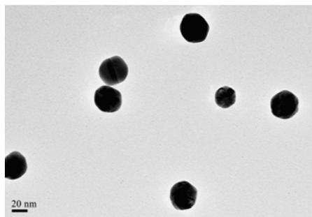
**Fig. S2** Typical TEM image of the as-prepared (+)AuNPs.
