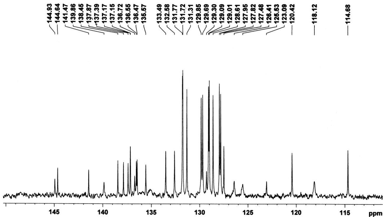
Figure S16.  $^{13}\text{C}$  NMR spectrum of compound 2 recorded in  $\text{CDCl}_3$  at room temperature.
