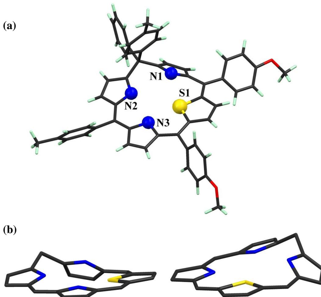
**Figure S21.** Single crystal X-ray structure of the compound **3**: (a) perspective view and (b) side view of compound **3** showing the distorted macrocyclic ring (*meso*-aryl rings and hydrogen atoms are omitted for clarity).
