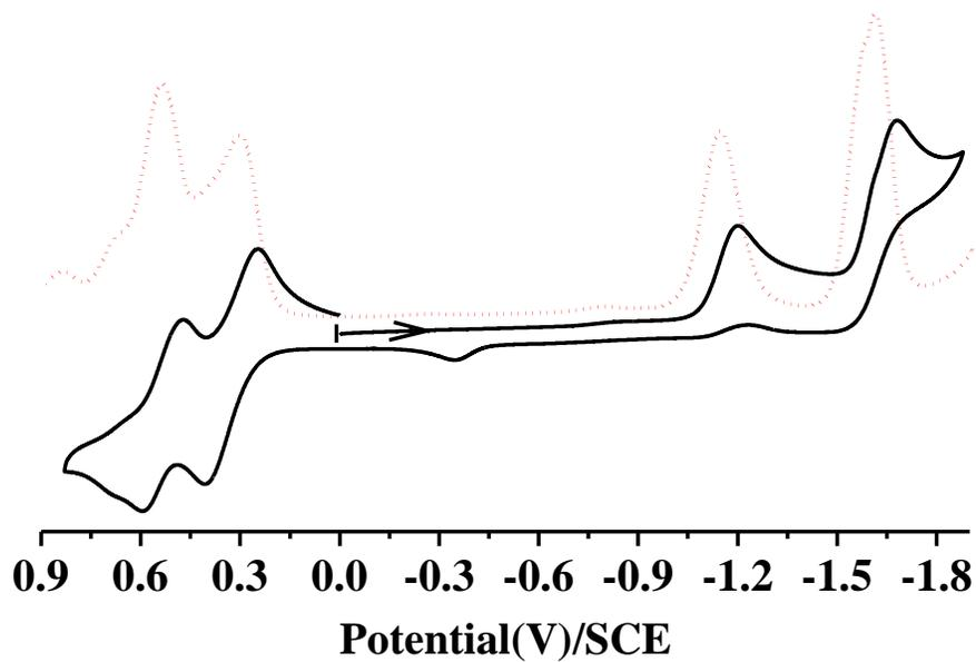
**Figure S20.** Redox waves of cyclic voltammograms along with differential pulse voltammograms of compound **3** recorded in  $\text{CH}_2\text{Cl}_2$  solvent using 0.1 M tetrabutylammonium perchlorate (TBAP) as supporting electrolyte and saturated calomel electrode (SCE) as reference electrode at scan rates of  $50 \text{ mVs}^{-1}$ .
