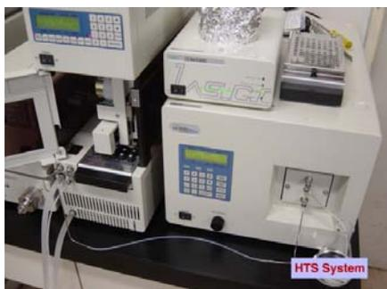
HTS system was constructed with an autosampler (JASCO AS-2057), a pump (JASCO PU-2080), and a CD-detector (JASCO CD-2095). A line between the auto sampler and the CD-detector was connected by Teflon tube as shown in the picture. For the CD-HTS examined in Figure 3 of the manuscript, the sample was prepared by a dilution of 25 μl of the reaction mixture with 950 μl of an eluent (iPrOH/Hex = 1/9). In each period of 3 min interval, 5 μl of the sample
